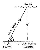
The light beam sweeps from the horizontal (angle x = 00) to the vertical (angle  $x = 90^{0}$ ). When the beam illuminates the base of the clouds directly above the detector, the angle x is read, and with d, the distance between the light source and the light source detector, known, the height of the clouds can be computed.
