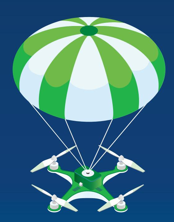
Some PARACHUTE SYSTEMS may contain pyrotechnics, CO2 cartridges, batteries or other materials that are considered DANGEROUS GOODS.
