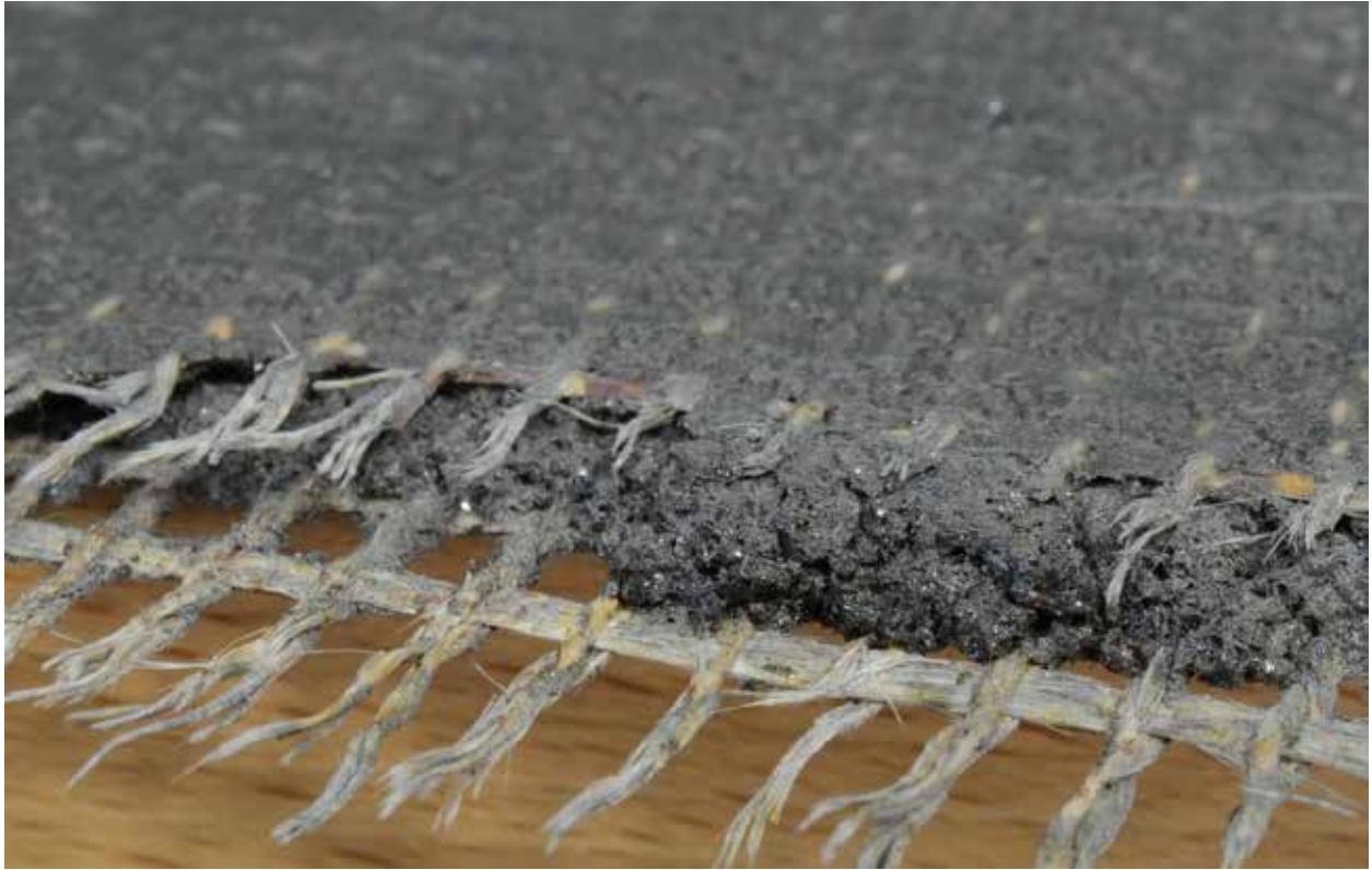
Figure C-12. Metal Saw Blade, CF24, Wet Cuts
