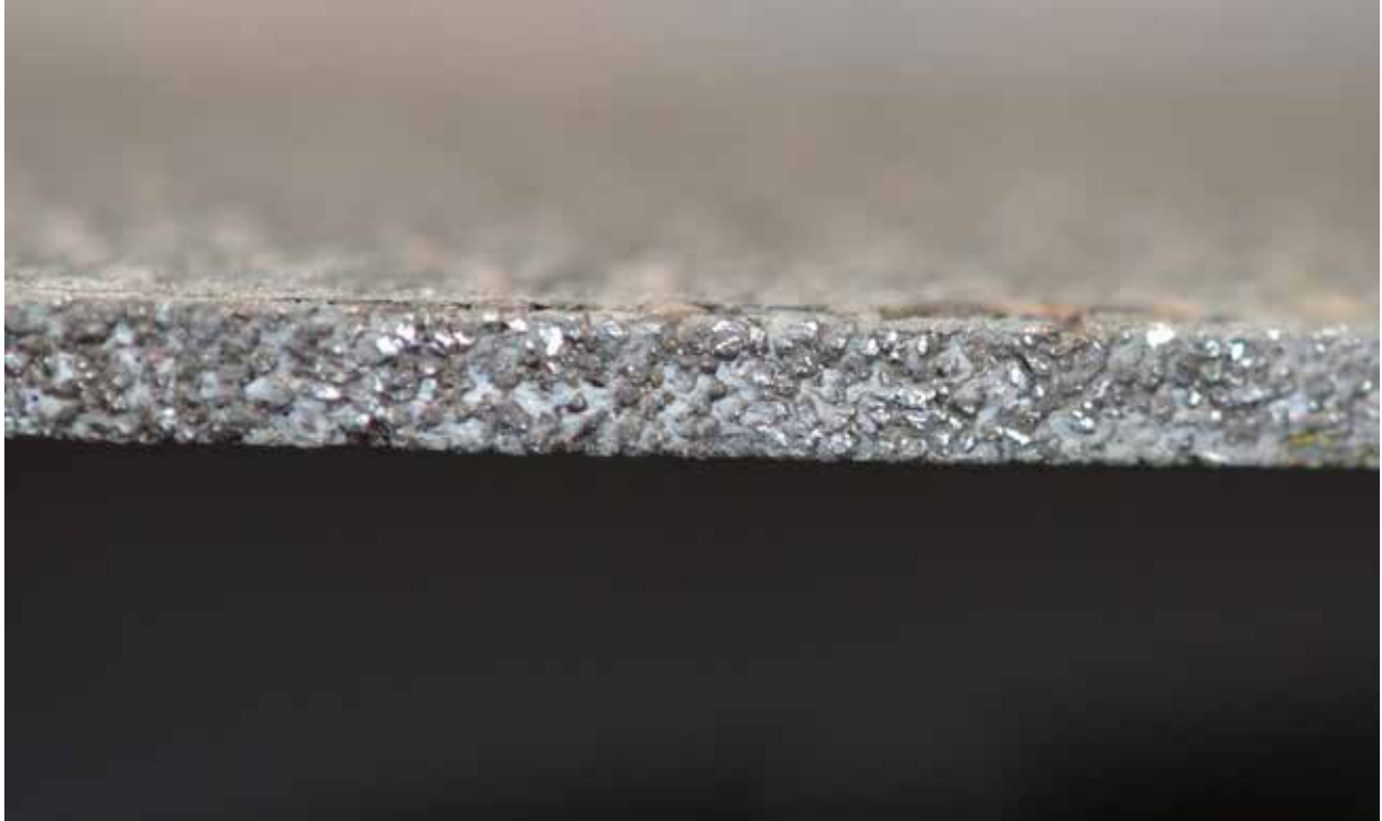
Figure C-8. Metal Saw Blade, G5, Wet Cuts
