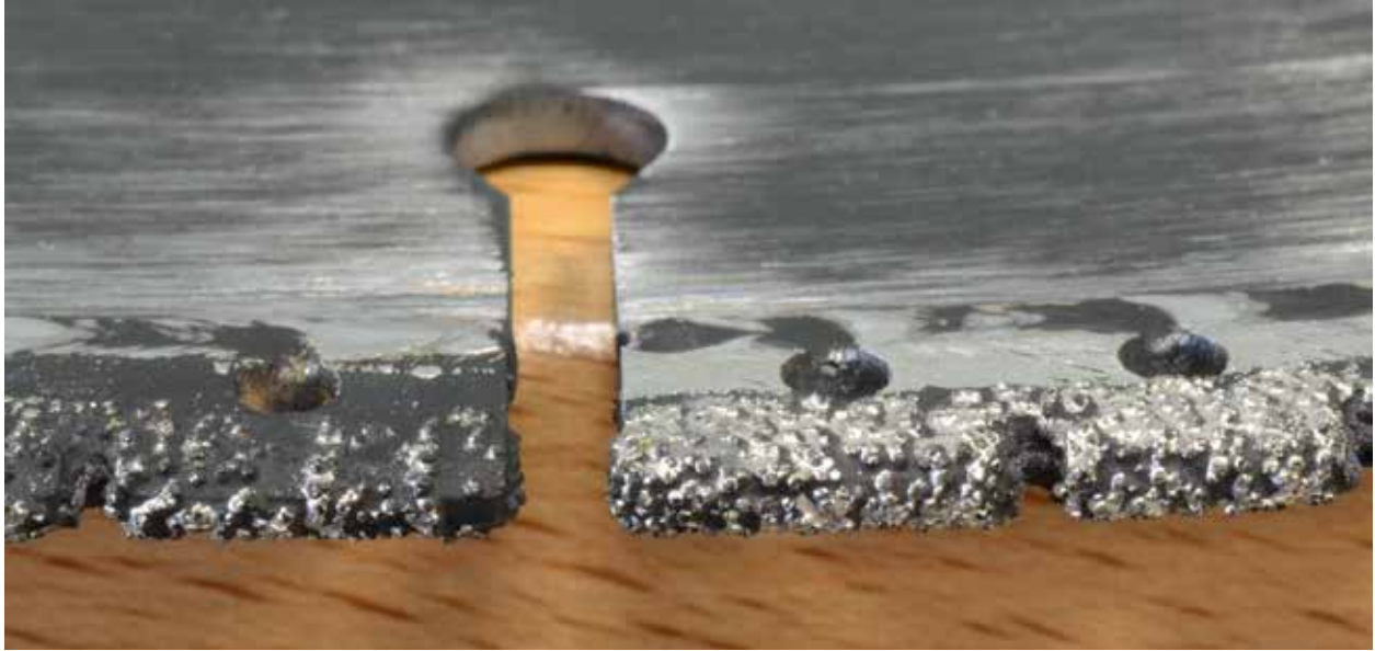
Figure C-34. Diamond Saw Blade, CF16, Wet Cuts
