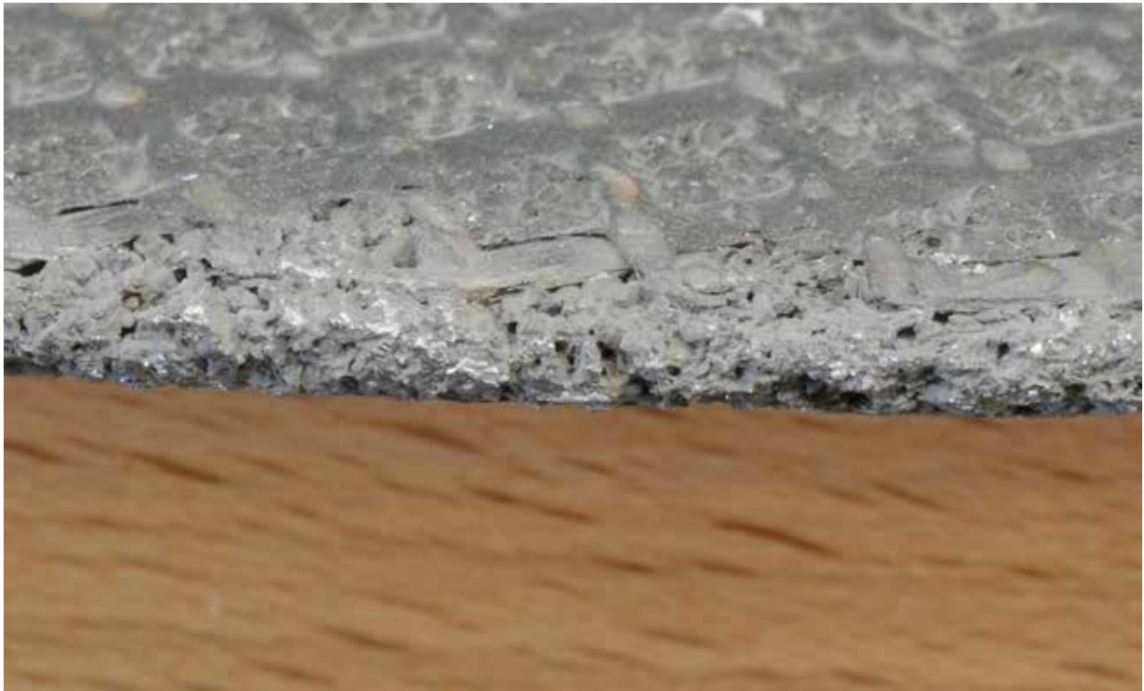
Figure C-17. Concrete Saw Blade, G3, Dry Cuts
