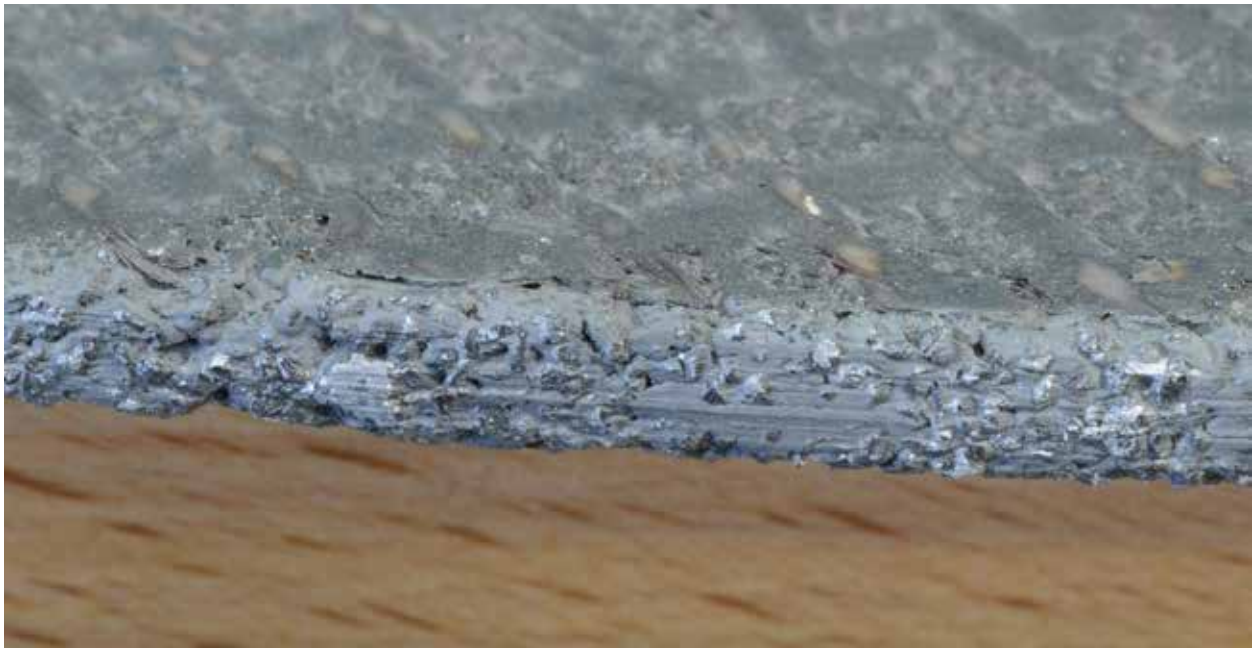
Figure C-5. Metal Saw Blade, G3, Dry Cuts
