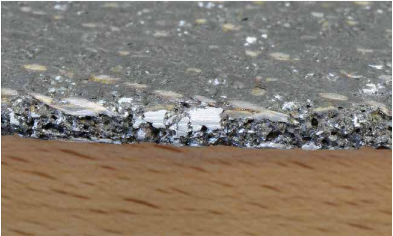
Figure C-1. Metal Saw Blade, AL06, Dry Cuts
