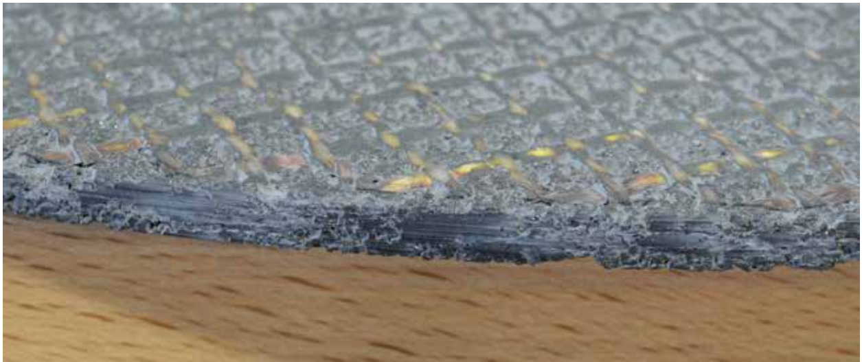
Figure C-9. Metal Saw Blade, CF16, Dry Cuts
