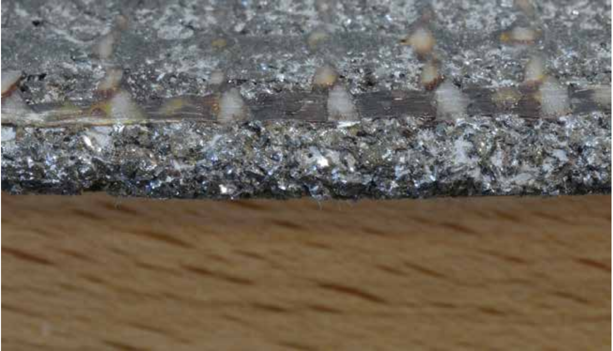
Figure C-18. Concrete Saw Blade, G3, Wet Cuts
