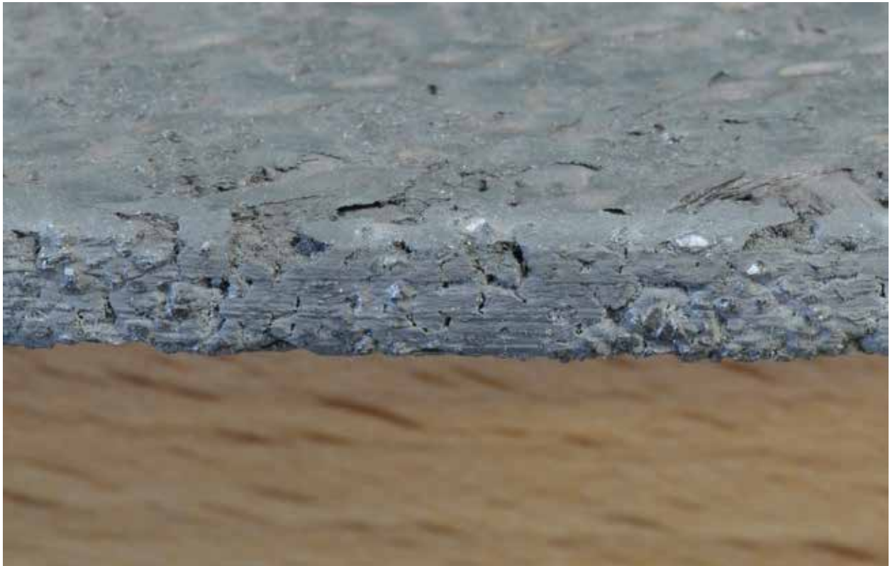
Figure C-7. Metal Saw Blade, G5, Dry Cuts
