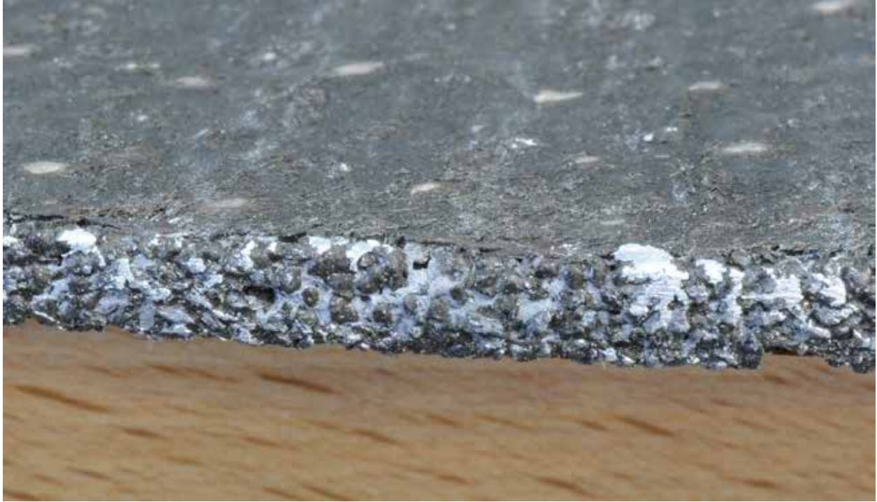
Figure C-6. Metal Saw Blade, G3, Wet Cuts
