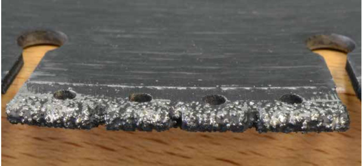
Figure C-30. Diamond Saw Blade, G3, Wet Cuts
