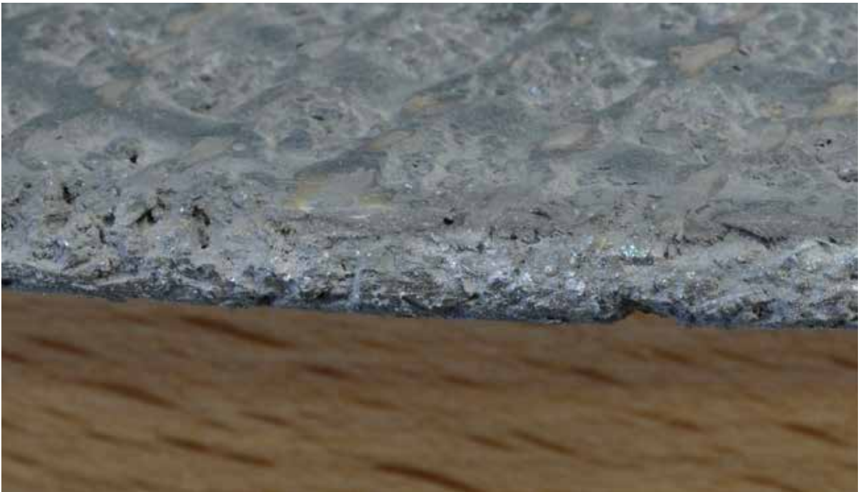
Figure C-19. Concrete Saw Blade, G5, Dry Cuts
