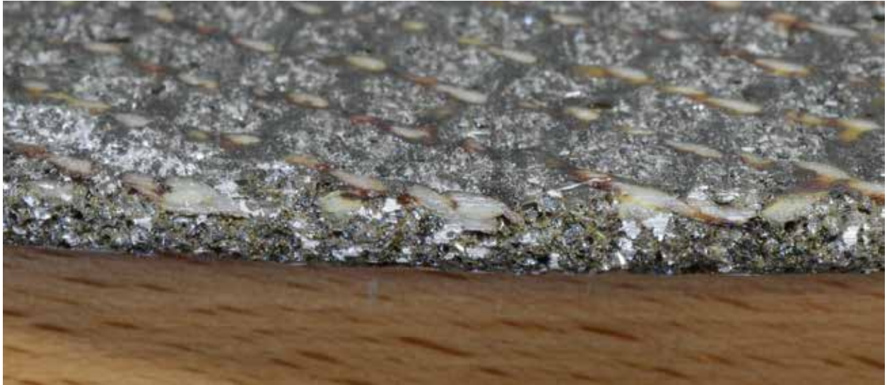
Figure C-16. Concrete Saw Blade, AL08, Wet Cuts
