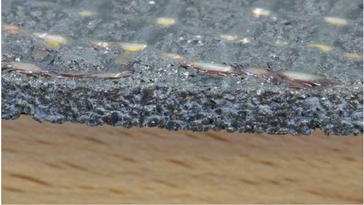
Figure C-10. Metal Saw Blade, CF16, Wet Cuts
