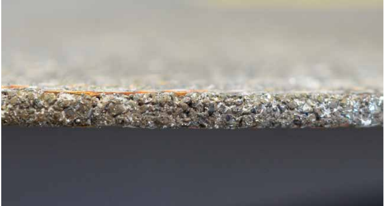
Figure C-20. Concrete Saw Blade, G5, Wet Cuts
