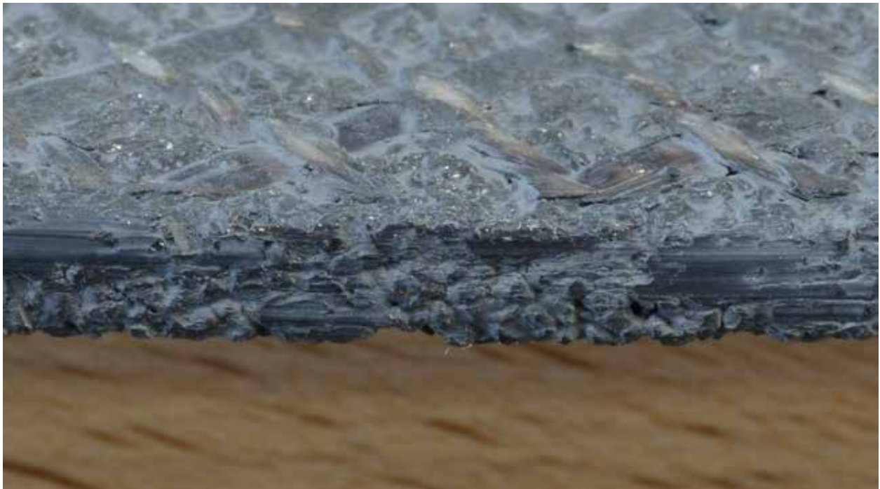
Figure C-11. Metal Saw Blade, CF24, Dry Cuts
