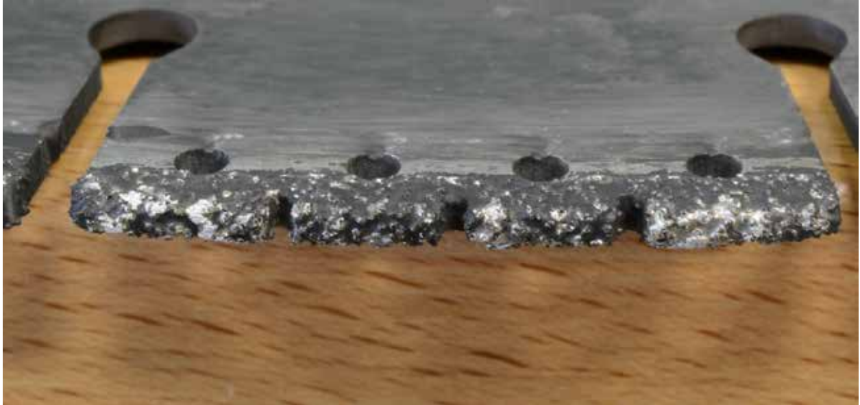
Figure C-25. Diamond Saw Blade, AL06, Dry Cuts
