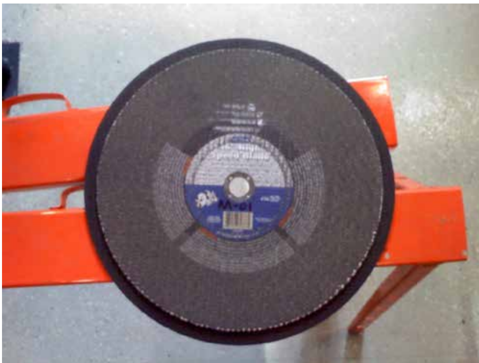
Figure 7. Metal Saw Blade Wear Following Practical Trials
