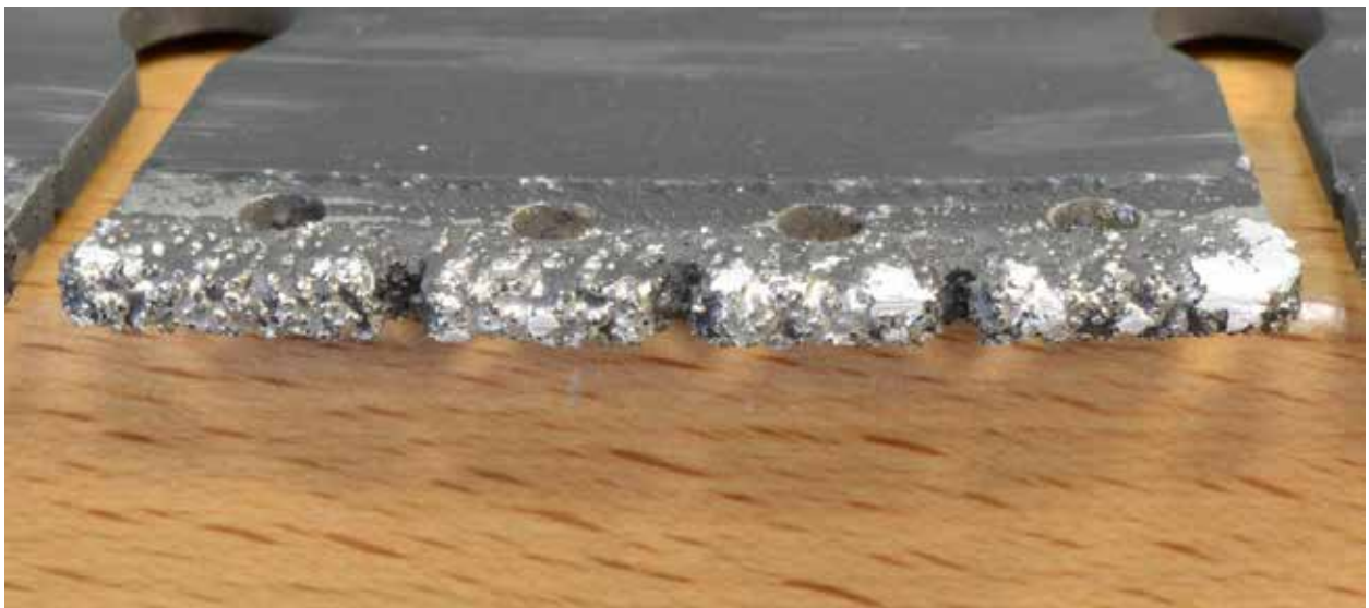
Figure C-27. Diamond Saw Blade, AL08, Dry Cuts
