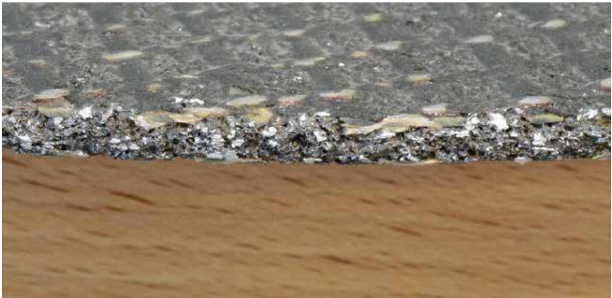
Figure C-15. Concrete Saw Blade, AL08, Dry Cuts
