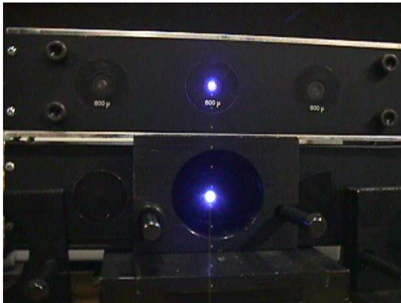
Figure 2. Light-Emitting Diode (top) and Incandescent (bottom) Enclosures
