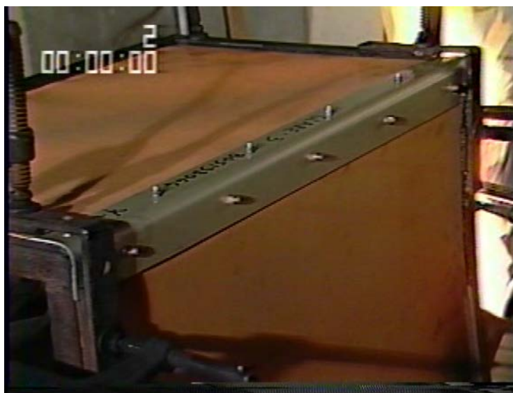
Figure 2. Cessna GLARE Cargo Liner Corner Test Setup
