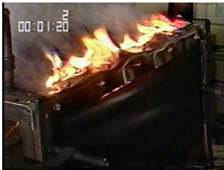
Figure 3. Cargo Liner Corner Test 2 of GLARE 3-3/2
