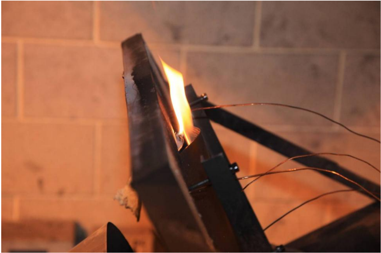
Figure 26. Chimney Effect in Test 6
