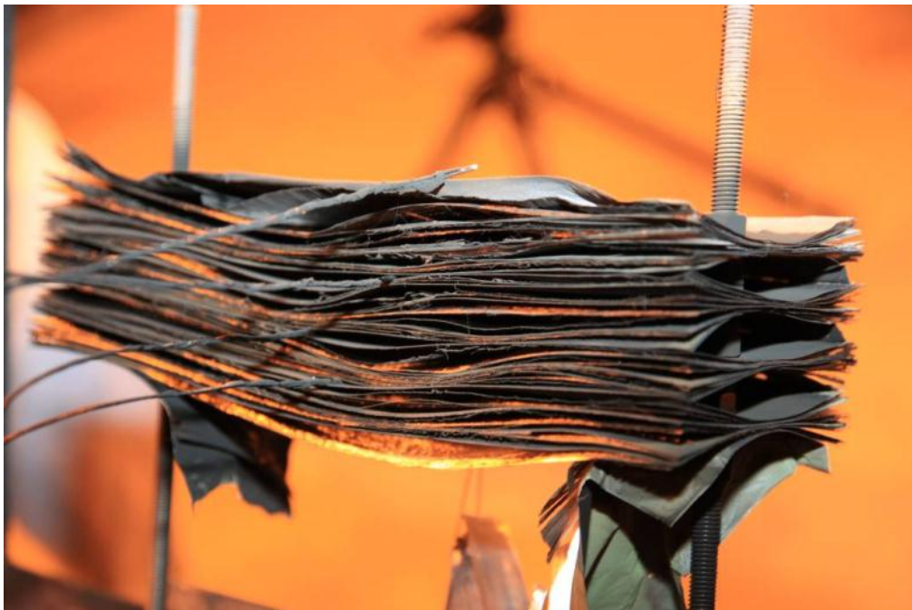
Figure 30. Delaminated Sample After Test 11
