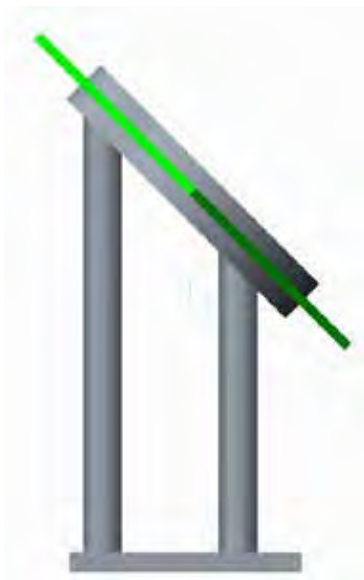
Figure A-2. The 45-Degree Angle Penetration Test Fixture Without Base Plate and Specimen
