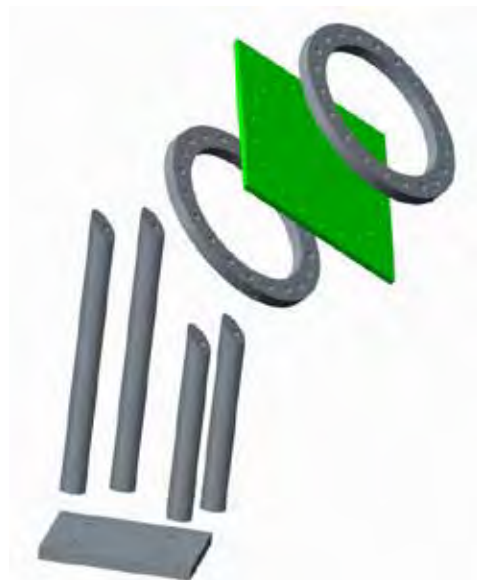
Figure A-2. The 45-Degree Angle Penetration Test Fixture Without Base Plate and Specimen
