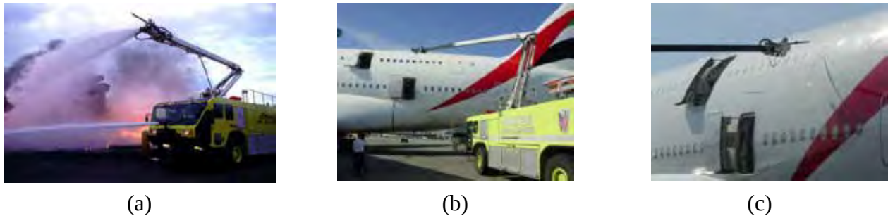
Figure 1. Views of an HRET Equipped With an ASPN in Operation [3]
