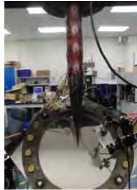
Figure 28. Setup of 45-Degree Angle Penetration Test With Strain Gage Installed Around the Boom
