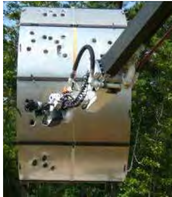
Figure 2. An ASPN Penetrating an Aluminum Alloy Panel Attached to a PAST [3]
