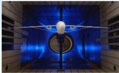
Transonic Truss-Braced Wing 5-10% fuel burn benefit
