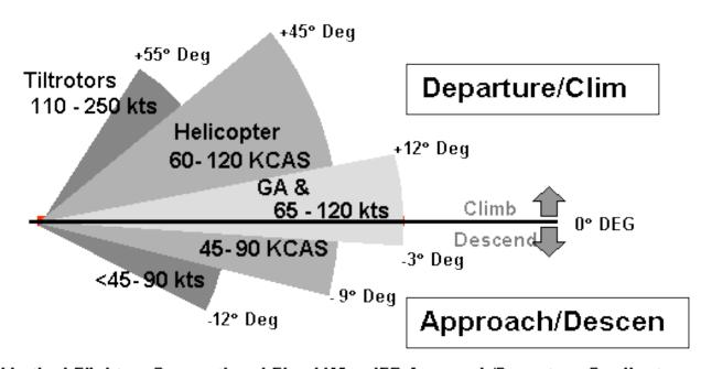
Vertical Flight vs Conventional Fixed Wing IFR Approach/Departure Gradient
