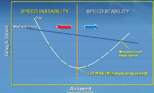
Figure 1 Airspeed vs. Drag in Level Flight
