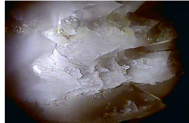
Ice crystal icing in ALF502 engine core flow path
