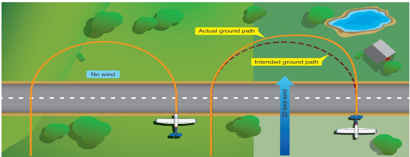
Figure 7-2. Effect of wind during a turn.
