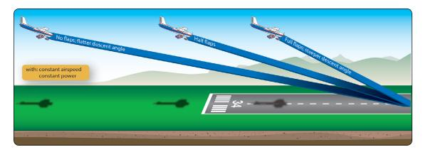
Figure 9-2. Effect of flaps on the approach angle.
