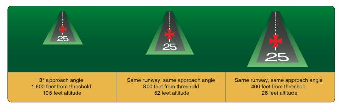
Figure 9-6. Runway shape during stabilized approach.
