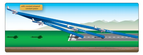
**Figure 9-1.** *Effect of flaps on the landing point.*
