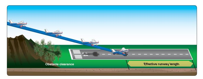
Figure 9-20. Landing over an obstacle.
