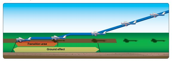
Figure 9-24. Soft/rough field approach and landing.
