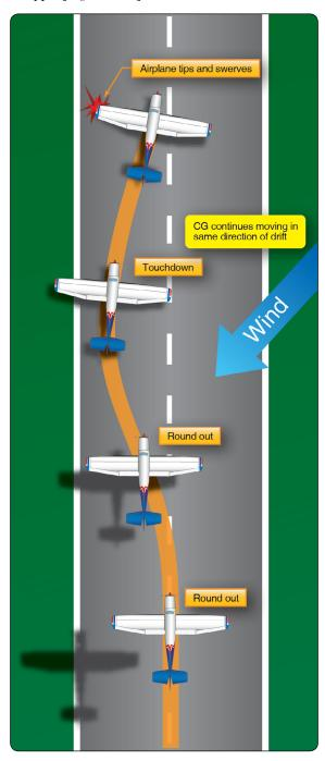
Figure 9-38. Start of a ground loop.
