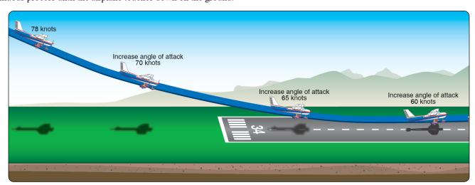
Figure 9-10. Changing angle of attack during round out.
