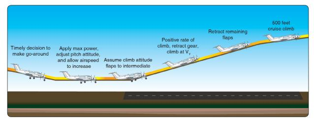
Figure 9-12. Go-around procedure.
