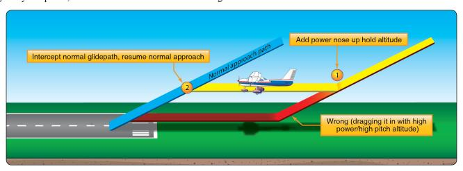
**Figure 9-30.** *Right and wrong methods of correction for low final approach.*
