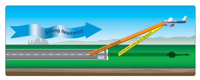
Figure 9-4. Effect of headwind on final approach.
