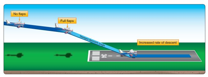
Figure 9-31. Change in glidepath and increase in descent rate for high final approach.
