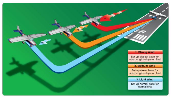
**Figure 9-25.** *Plan the base leg for wind conditions.*
