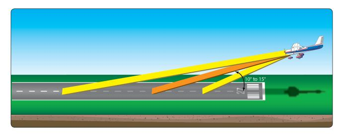
**Figure 9-9.** To obtain necessary visual cues, the pilot should look toward the runway at a shallow angle.
