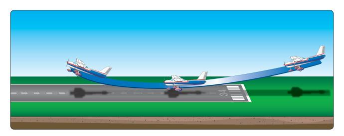
Figure 9-34. Ballooning during roundout.
