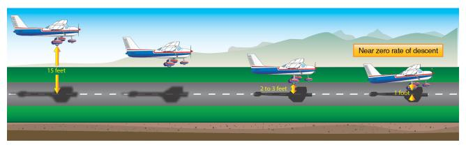
**Figure 9-11.** A well-executed round out results in attaining the proper landing attitude.
