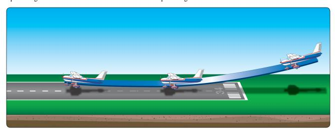
Figure 9-33. Floating during round out.
