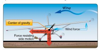
Figure 9-37. Drifting during touchdown.
