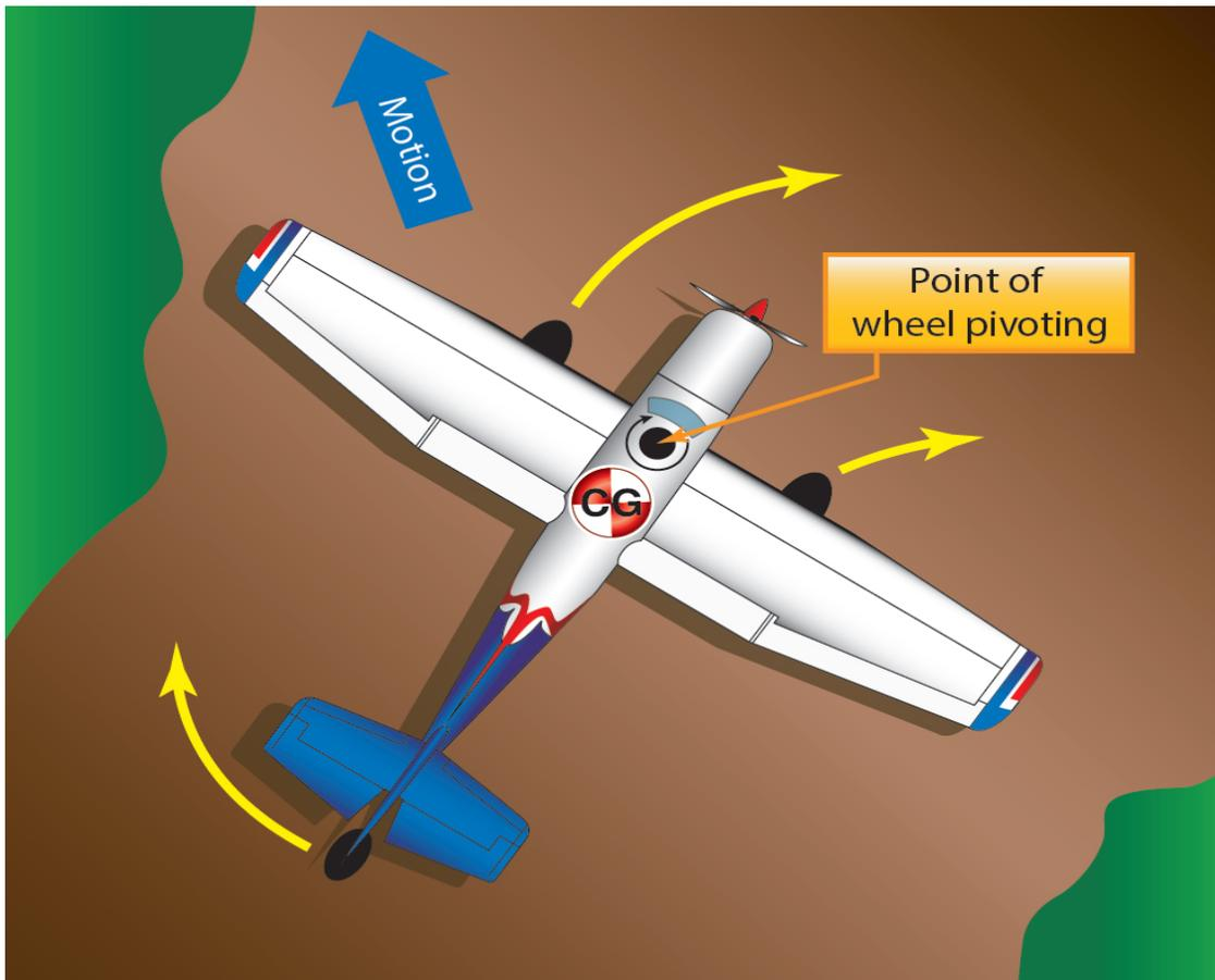
**Figure 14-4.** *Effect of CG on directional control.*
