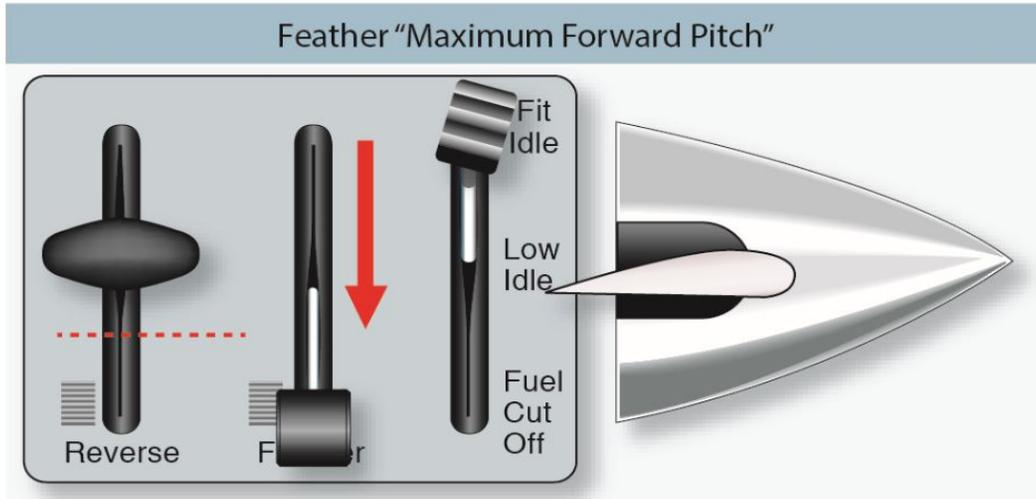
Figure 15-8C. Propeller feather (maximum forward pitch angle) characteristics.
