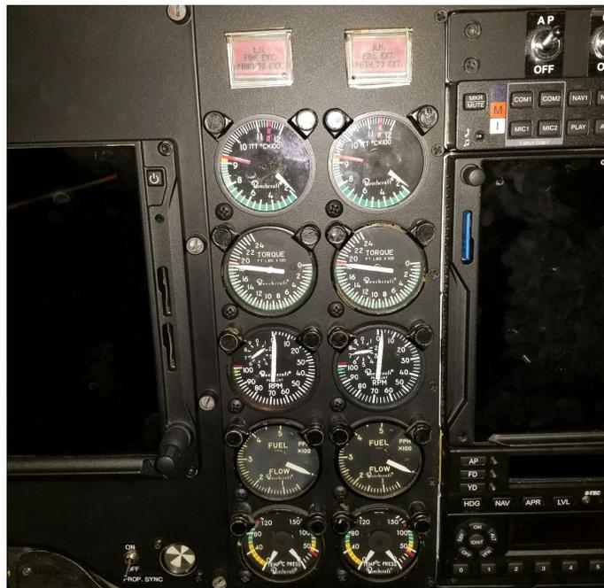
Figure 15-4. Powerplant instrumentation—fixed-shaft turboprop engine.
