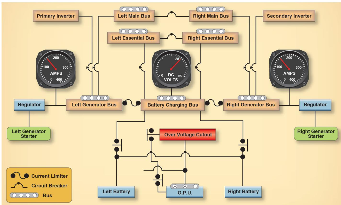
Figure 15-10. Simplified schematic of turboprop airplane electrical system.
