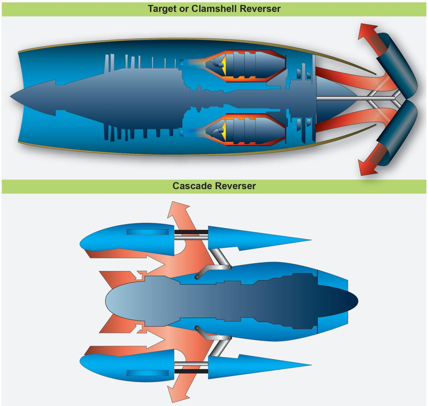
Figure 16-11. Thrust reversers.
