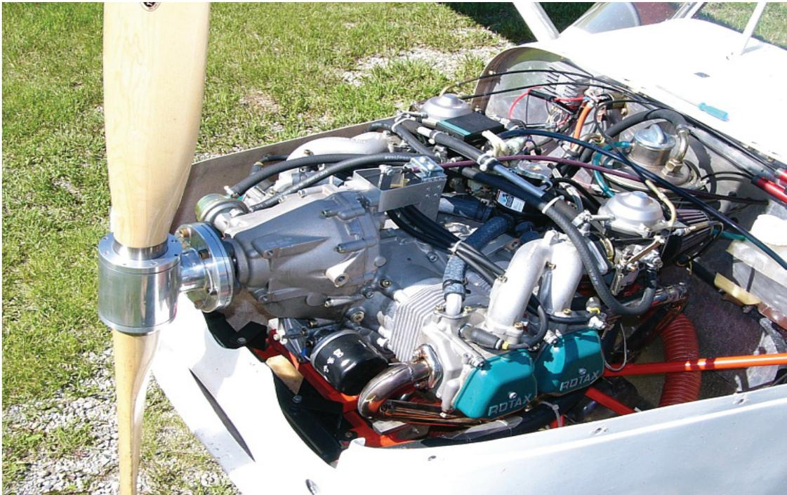
Figure 17-4. A water-cooled 4-cycle engine.
