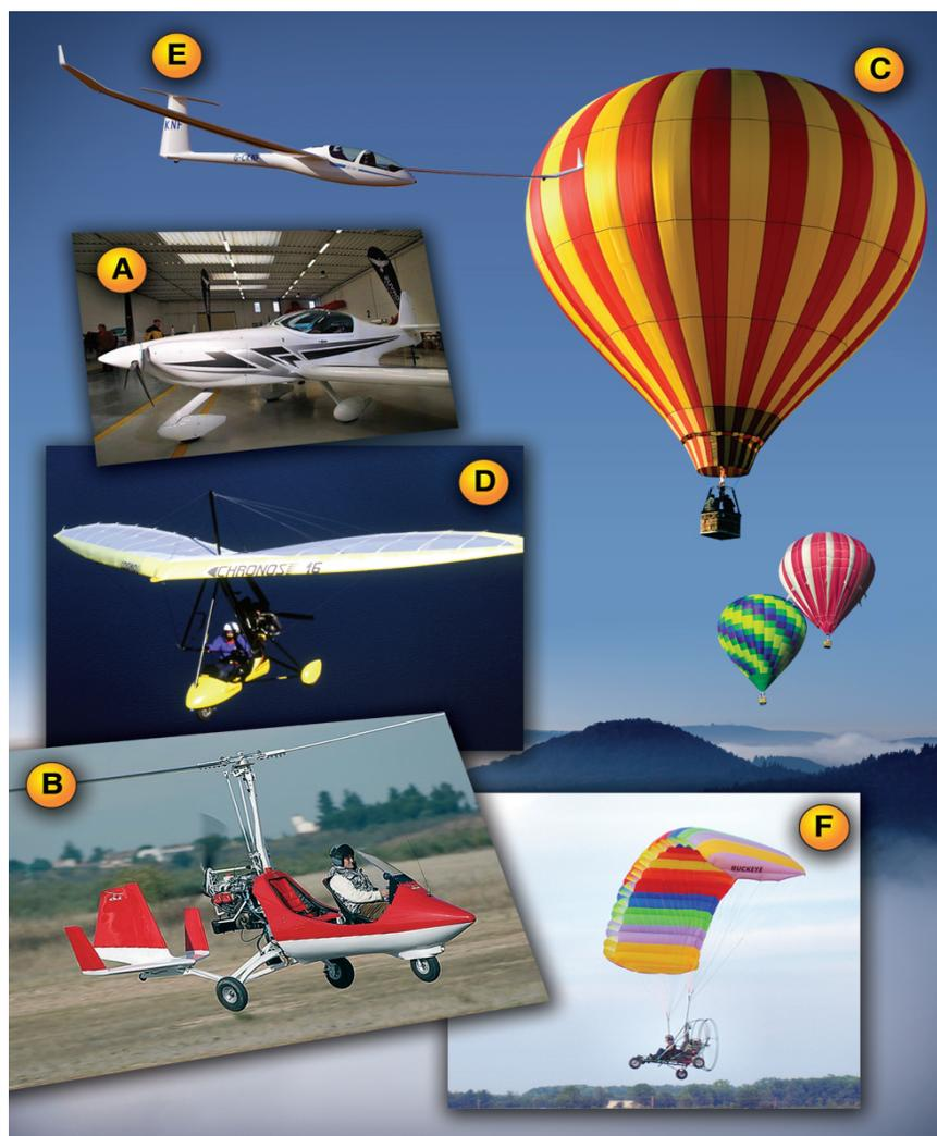
**Figure 17-1.** The LSA category covers a wide variety of aircraft including: A) airplane, B) gyroplane, C) lighter-than-air, D) weight-shift-control, E) glider, and F) powered parachute.
