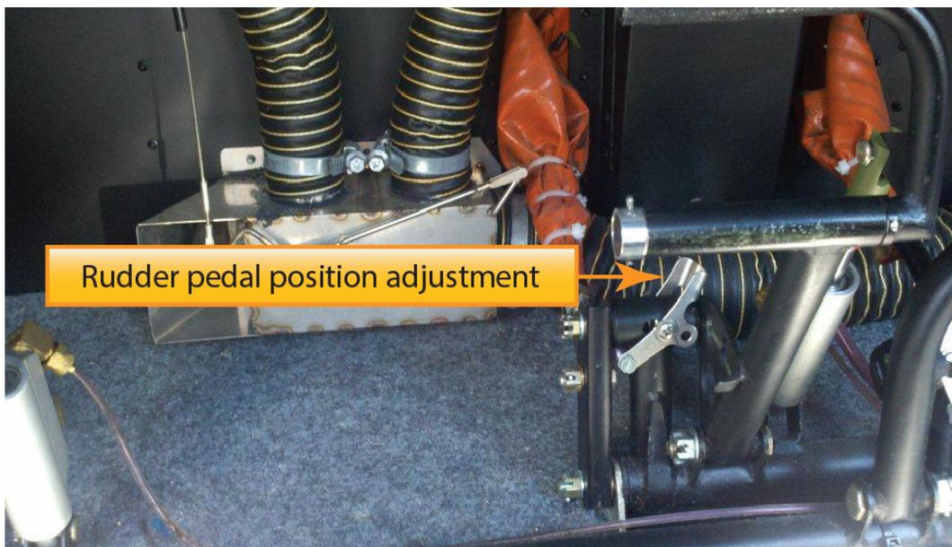
Figure 17-10. Adjustment lever for the rudder pedal position.
