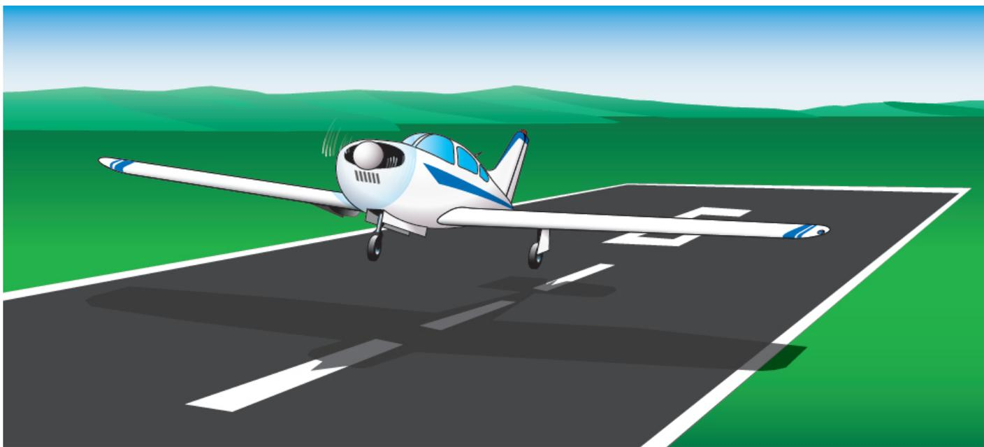
**Figure 18-7.** *Landing with one main gear retracted.*
