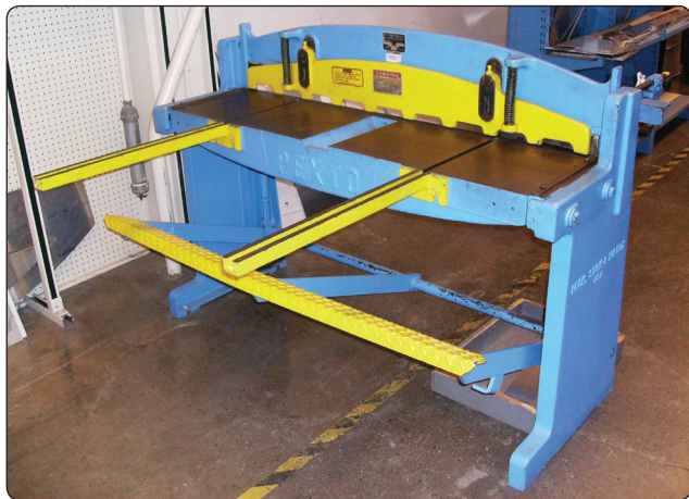
Figure 4-24. Foot-operated squaring shear.
