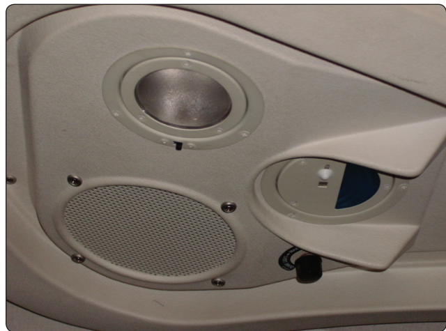
Figure 9-181. Interior cockpit and cabin light system.
