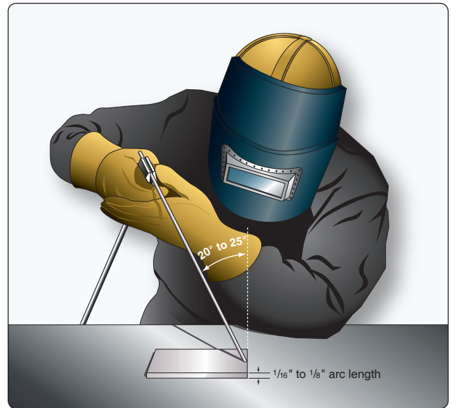
Figure 5-32. Angle of electrode.
