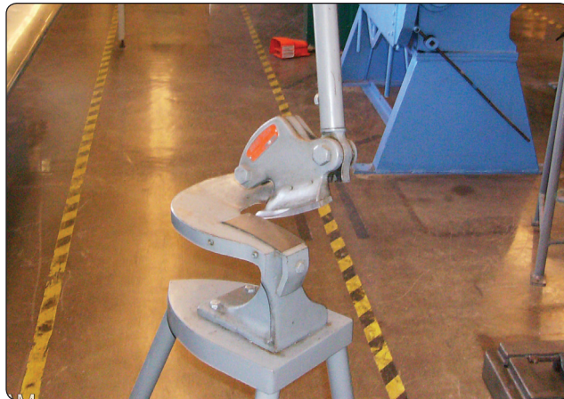
Figure 4-25. Throatless shears.
