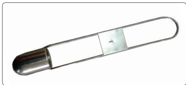
Figure 8-10. A Zahn cup viscosity measuring cup.
