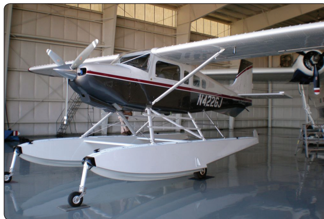
Figure 1-85. Retractable wheels make this aircraft amphibious.
