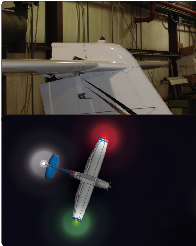
Figure 9-177. Anticollision lights.
