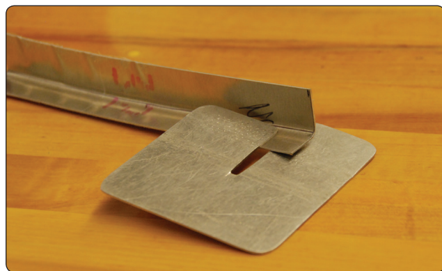
Figure 4-164. Samples of joggled metal.
