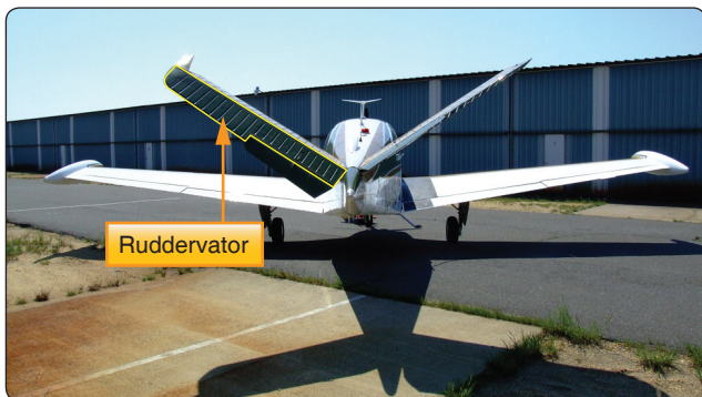
Figure 1-59. Ruddervator.
