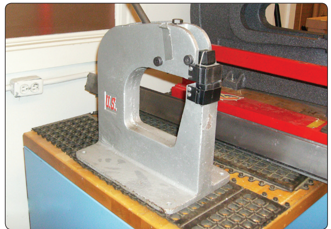
Figure 4-67. Hand-operated shrinker and stretcher unit.
