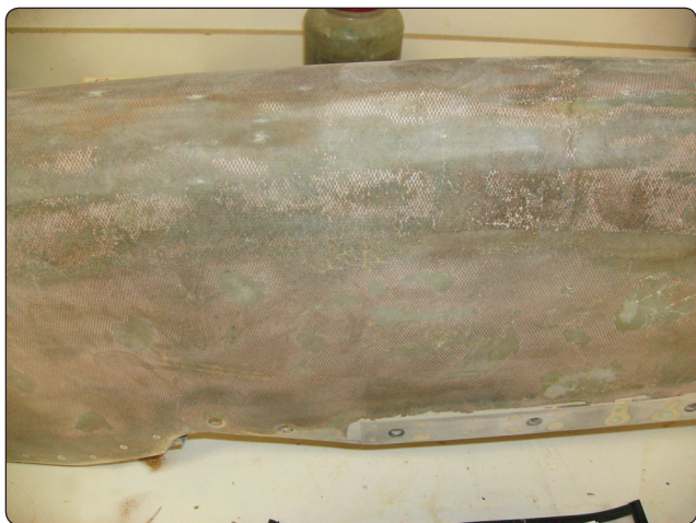
Figure 7-8. Copper mesh lightning protection material.
