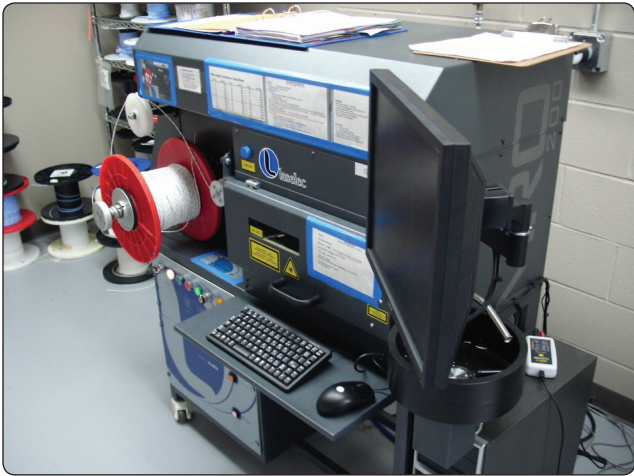
Figure 9-126. Laser wire printer.
