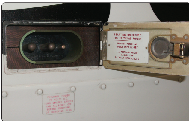
Figure 9-89. External power receptacle.
