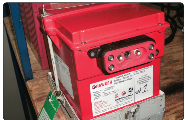
Figure 9-33. Valve-regulated lead-acid battery (sealed battery).
