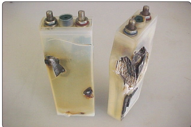
Figure 9-35. Thermal runaway damage.
