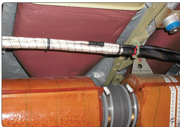
Figure 9-113. Shielded wire harness for flight control.
