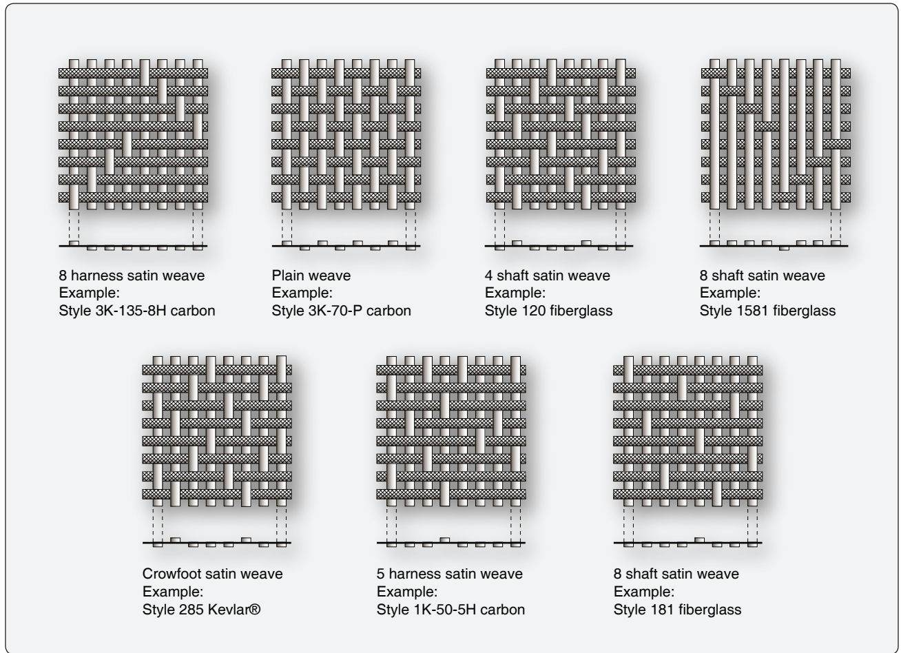
Figure 7-5. Typical fabric weave styles.
