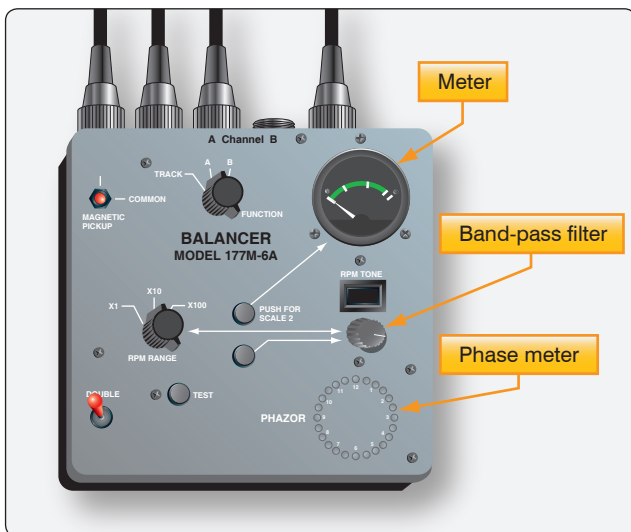
Figure 2-52. Balancer/Phazor.
