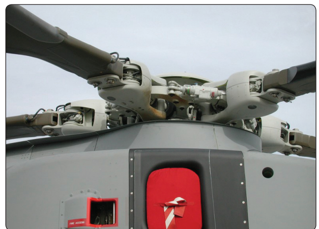
Figure 1-99. Five-blade articulated main rotor with elastomeric bearings.
