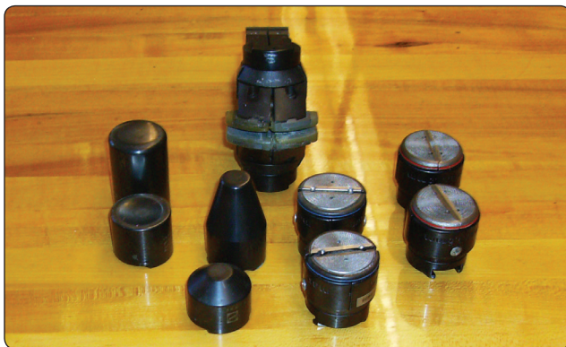
Figure 4-66. Shrinking and stretching tools.
