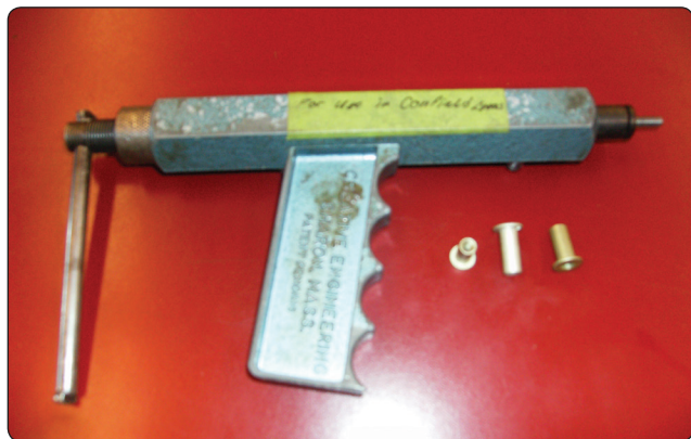
Figure 4-113. Rivet nut installation.
