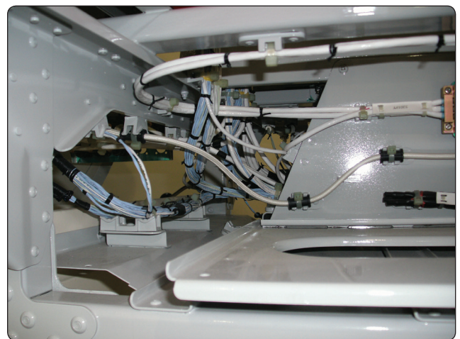
Figure 9-134. Drip loop.
