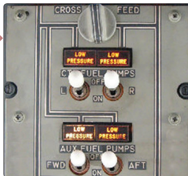
Figure 14-87. A transport category aircraft fuel panel with low pressure warning lights for each fuel boost pump.
