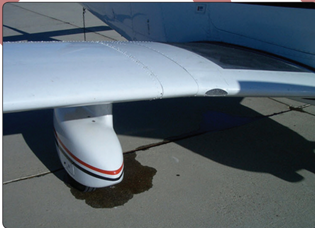
Figure 13-120. The cause of all aircraft brake leaks must be investigated, repaired, and tested before releasing the aircraft for flight.
