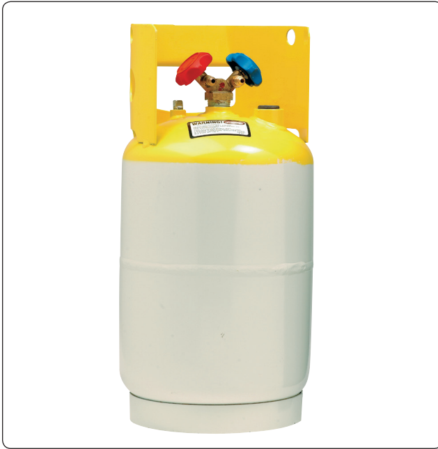
Figure 16-89. A 30 pound R134a refrigerant container with dual fittings. The fitting controlled by the blue valve wheel opens to the vapor space above the liquid refrigerant for connection to the low side of the vapor cycle system. The fitting controlled by the red valve wheel draws liquid refrigerant from the bottom of the cylinder through a stand tube. This fitting is connected to the system high side. On containers without dual fittings, the container must be inverted to deliver liquid refrigerant through a connected hose.
