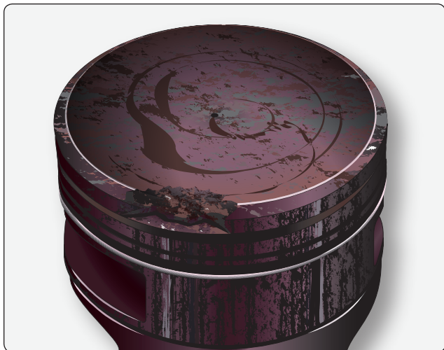
Figure 14-7. Preignition can cause detonation and damage to the engine.
