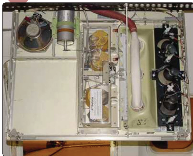
Figure 16-29. An oxygen generator mounted in place in an overhead passenger service unit of an air transport category aircraft.
