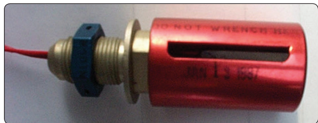
Figure 14-103. A float switch installed in a fuel tank can close the refueling valve when the tanks are full during pressure fueling of an aircraft. Other more sophisticated automatic shutoff systems exist.
