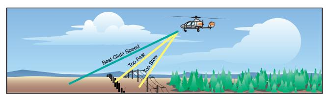
Figure 21-3. Any deviation from best glide speed will reduce the distance you can glide and may cause you to land short of a safe touchdown point.
