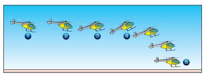
Figure 10-3. Rapid deceleration or quick stop.
