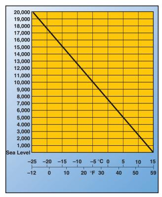
Figure 20-6. Standard temperature chart.
