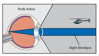
Figure 13-4. In low light, the cones lose much of their visual acuity, while rods become more receptive. The eye sacrifices sharpness for sensitivity. Your ability to see an object directly in front of you is reduced, and you lose much of your depth perception, as well as your judgment of size.
