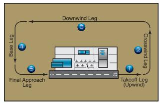
Figure 9-18. A standard traffic pattern has turns to left and five designated legs.
