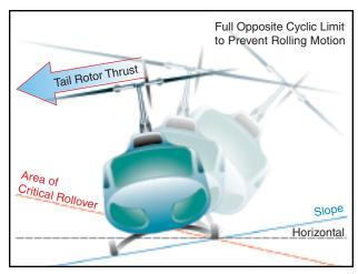
Figure 11-7. Upslope rolling motion.
