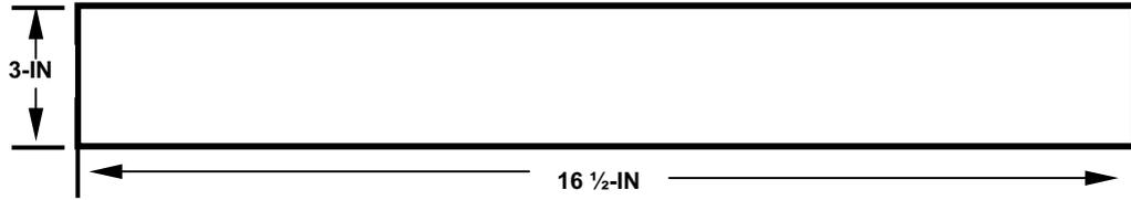
3. On the 3-inch length, fold ends under ½-inch and sew with a light-duty sewing machine, type 301, and size E nylon thread, 7 to 11 stitches per inch. Backstitch not less than ½-inch.
