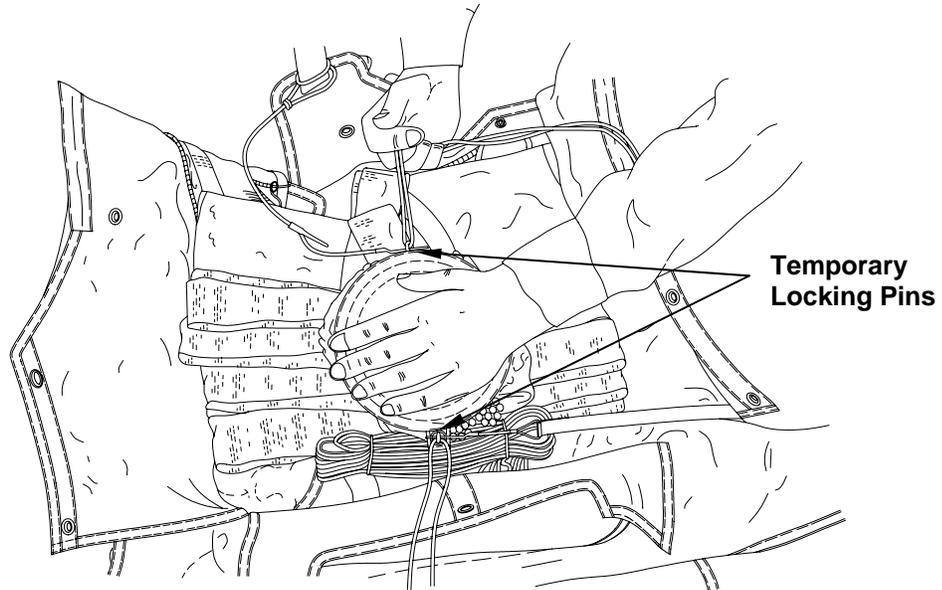
12. Route pull-up cord through grommet in bottom flap. Pull up closing loop and reinsert temporary locking pin.
