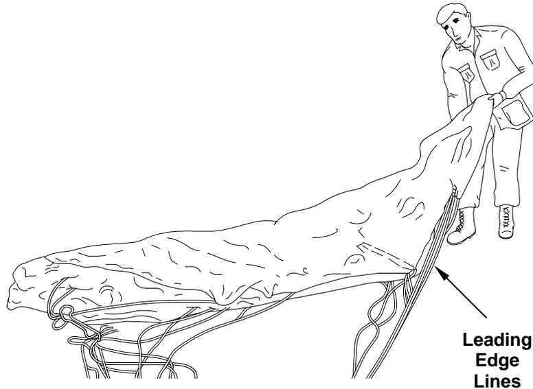
3. Remove any twists, turns, and tangles between suspension line groups.
