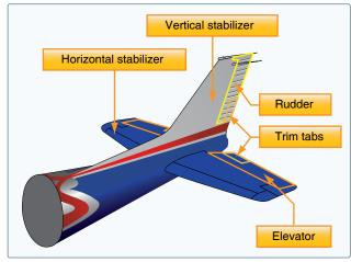
Figure 3-10. Empennage components.
