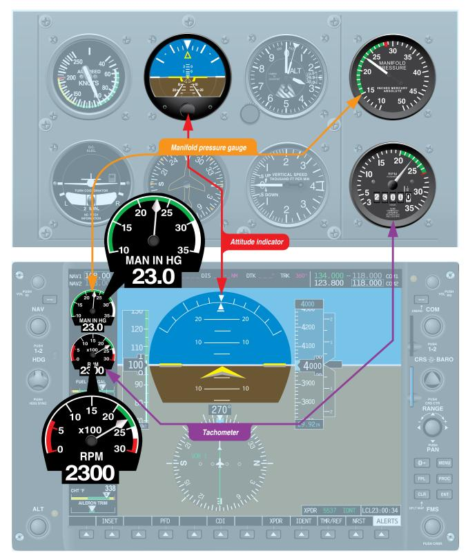
Figure 3-20. Control instruments.
