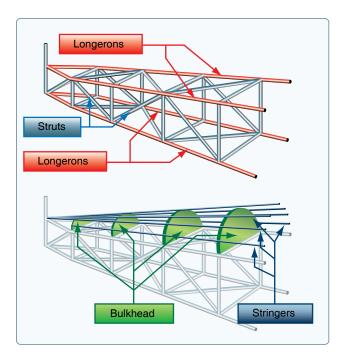
**Figure 3-5.** *Truss-type fuselage structure.*
