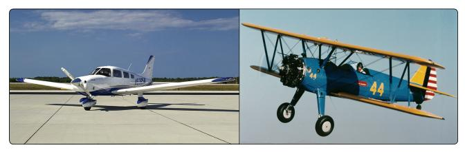
Figure 3-6. Monoplane (left) and biplane (right).
