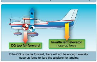
**Figure 3-3.** *Center of gravity (CG).*
