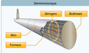
Figure 3-14. Semimonocoque and monocoque fuselage design.
