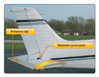
Figure 3-11. Stabilator components.
