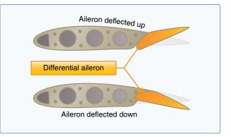
Figure 6-6. Differential ailerons.
