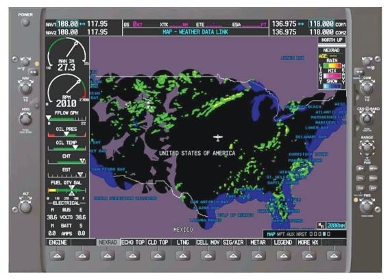
Figure 13-17. NEXRAD radar display.
