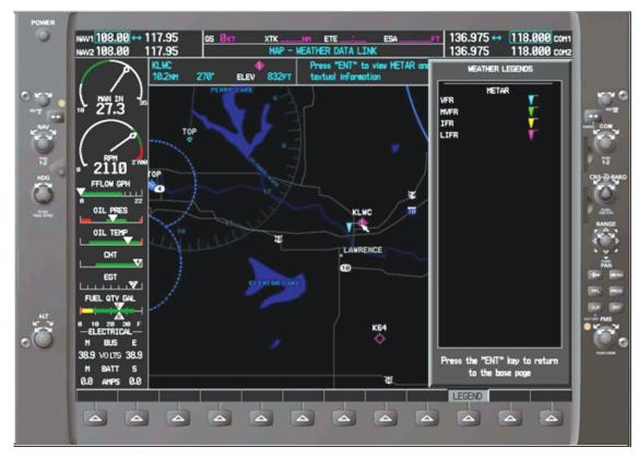
Figure 13-21. Graphical METAR legend display.
