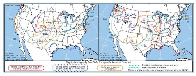
Figure 13-13. Significant weather prognostic chart.
