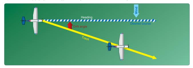
Figure 16-15. Effects of wind drift on maintaining desired course.
