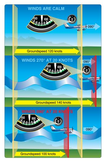
**Figure 16-13.** *Motion of the air affects the speed with which aircraft move over the Earth's surface. Airspeed, the rate at which an aircraft moves through the air, is not affected by air motion.*
