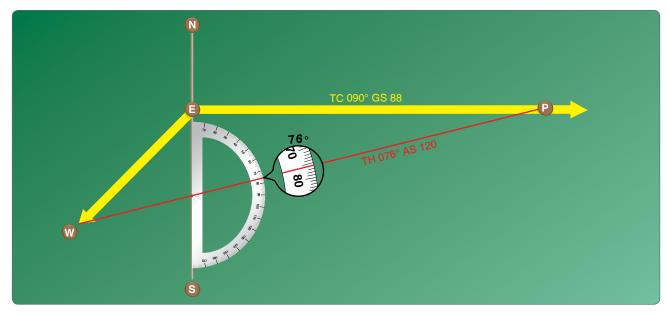
Figure 16-22. Finding true heading by the wind correction angle.
