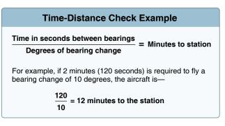
Figure 16-33. *Time-distance check example.*
