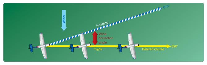
Figure 16-17. Establishing a wind correction angle that counteracts wind drift and maintains the desired course.
