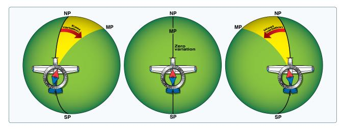
Figure 16-10. Effect of variation on the compass.
