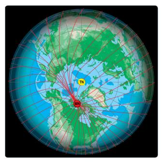
**Figure 16-8.** Magnetic meridians are in red while the lines of longitude and latitude are in blue. From these lines of variation (magnetic meridians), one can determine the effect of local magnetic variations on a magnetic compass.
