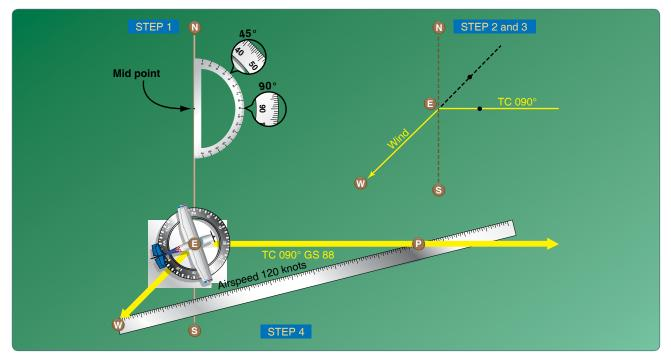
Figure 16-21. Steps in drawing the wind triangle.
