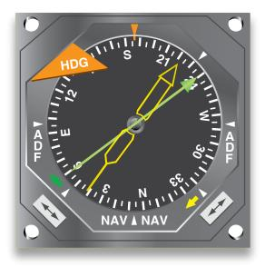
Figure 16-31. Radio magnetic indicator.
