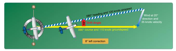
Figure 16-19. Principle of the wind triangle.
