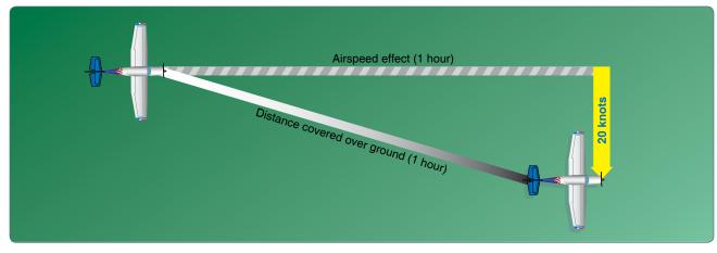
Figure 16-14. Aircraft flight path resulting from its airspeed and direction and the wind speed and direction.
