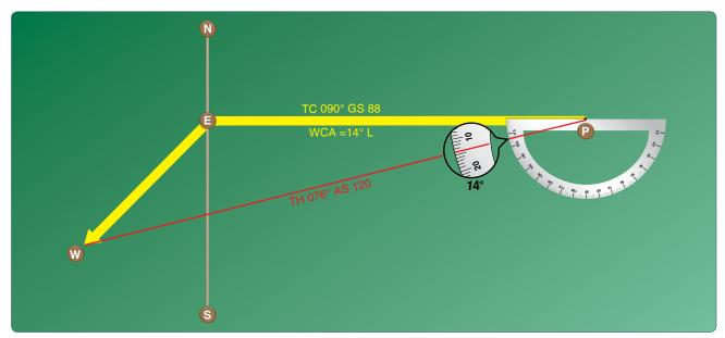
Figure 16-23. Finding true heading by direct measurement.
