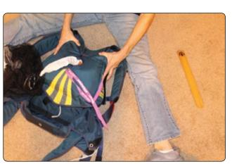
**Figure 5-152.** *S*-fold bridle and evenly distribute on both sides of container.
