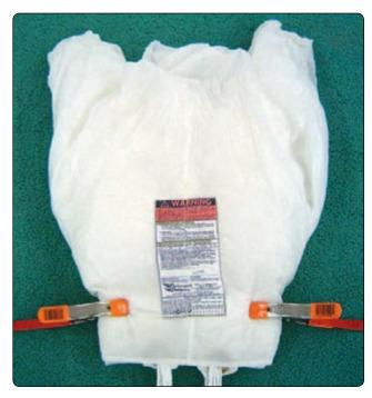
Figure 5-93. Wrap tail, two clamps.
