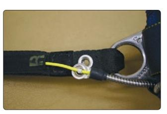
Figure 4-46. 3-ring cable through loop.
