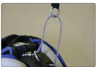
Figure 2-59. RSL lanyard extension.
