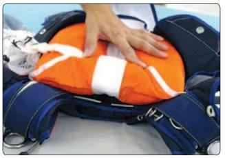
Figure 5-106. Fold the yoke over the bridle.
