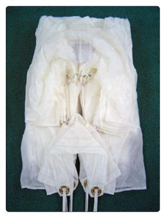
Figure 5-89. Fold tail back for wind channel.
