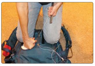
**Figure 5-161.** *Pull top closing loop through the grommet and insert pin.*
