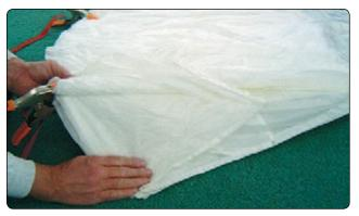
Figure 5-76. Fold half under "A" lines.
