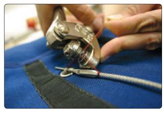
Figure 5-68. Compressing the seal.
