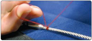
Figure 5-65. Lark's head the thread on the cable.
