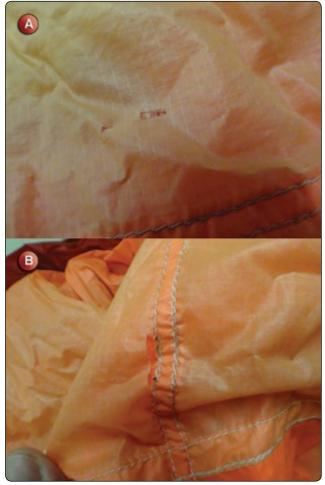
Figure 7-10. Fabric damage.
