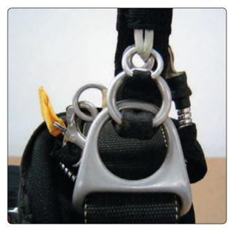
Figure 5-26. 3-Ring<sup>®</sup> release system.
