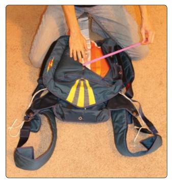
Figure 5-149. Close either side flap (not side-sensitive).
