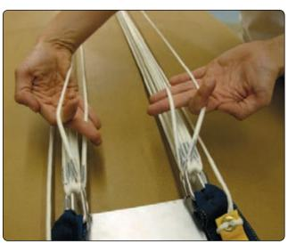
Figure 5-9. Round canopy—four-line check at four-link system.
