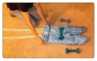
**Figure 5-132.** The length and width of the S-fold is determined by the width of the container and the distance between the main/reserve vertical partition and the bottom flap grommet.
