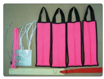
Figure 5-31. Round parachute packing tools.
