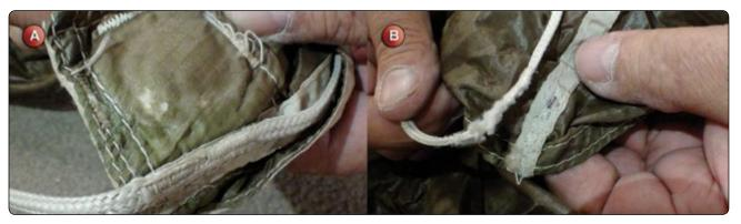
Figure 7-6. Stabilizer damage.
