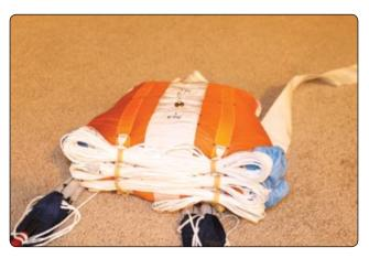
**Figure 5-142.** *Insert a bodkin through the channel in the bag where the hemostats were.*
