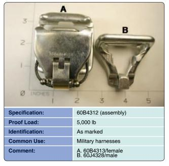
Figure 3-70. Release, parachute canopy quick disconnect, Capewell.
