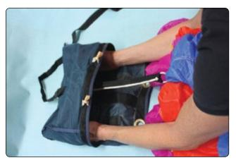
**Figure 4-18.** *The "cocoon" should be slightly wider than the deployment bag.*
