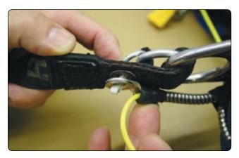
Figure 4-45. 3-ring housing terminal over loop (rear).
