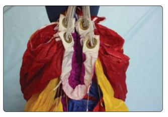
**Figure 4-12.** *The slider can be quartered or simply halved with the slider grommets resting up against the slider stops at the stabilizers.*
