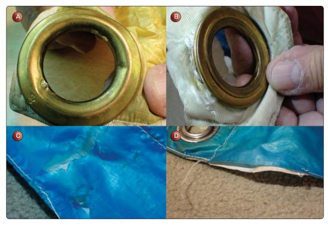
Figure 7-3. Slider damage.
