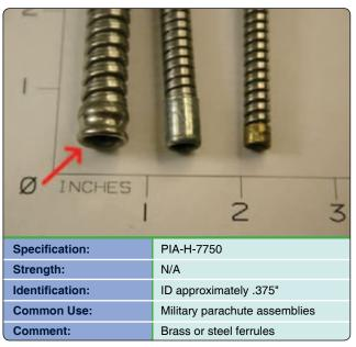
Figure 3-95. Housing, flexible, ripcord.
