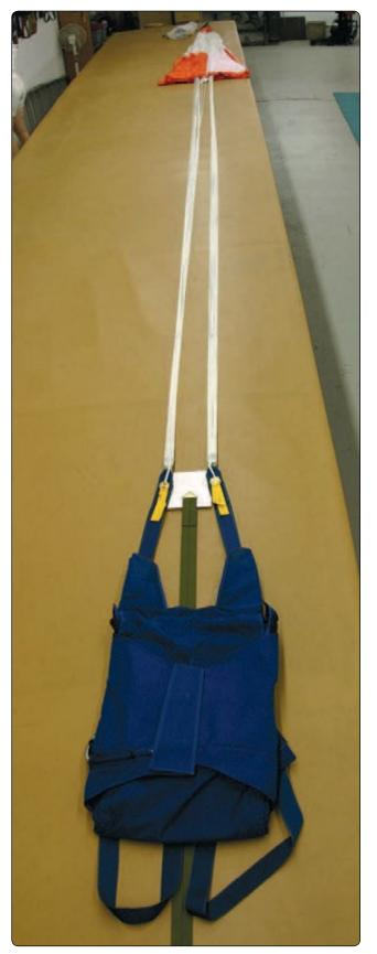
Figure 5-32. Round parachute assembly on packing table.
