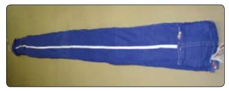
Figure 2-26. *Type 6 deployment—Sleeve*.
