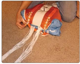
**Figure 5-138.** *Use the flaps of the bag to control the canopy and help push it into the bag.*
