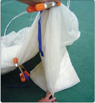
Figure 5-78. *Hold "B" clamp vertically over "A" clamp.*
