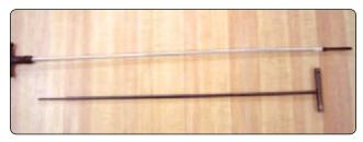
Figure 6-23. Pilot chute threading tool.
