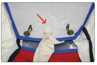
Figure 2-11. Square reserve hesitator loop configuration.
