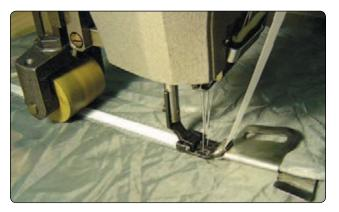
Figure 6-85. Tape feeder and French seam folder.
