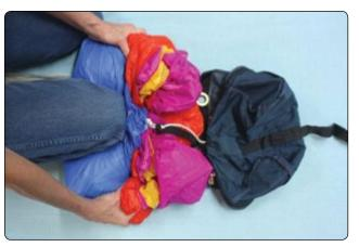
**Figure 4-24.** *Most canopies take two S folds. Pull PCA ring outward so that it is up against the grommet inside the bag.*
