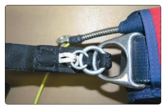
Figure 4-43. 3-ring loop over the top ring.
