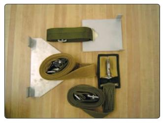
Figure 6-51. Tension board assembly with apex tiedown.
