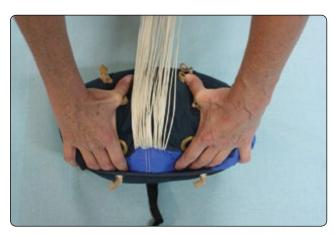
Figure 4-28. Use the flap of the bag to help control the canopy.
