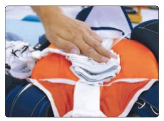
Figure 5-105. "S" fold the bridle on bag.
