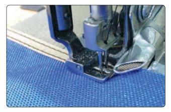
Figure 6-82. Material with binding tape.
