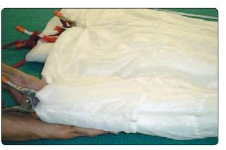
Figure 5-77. Smooth panels under "A" lines.
