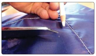
Figure 7-23. Cutting out damaged area.
