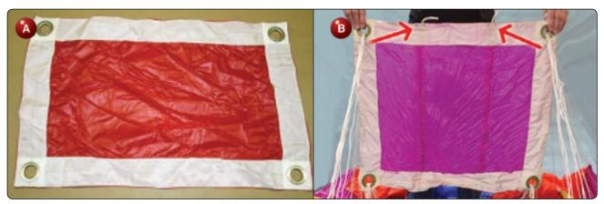
Figure 2-20. A) Non-collapsible slider and B) collapsible slider.
