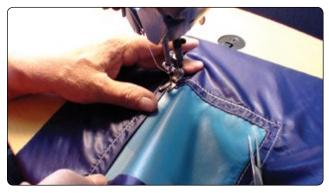
Figure 7-27. Correct fold corner seam.
