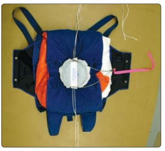
Figure 5-62. Pilot chute seated in position.
