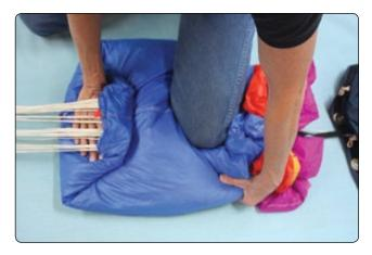
Figure 4-21. Make the first "S" fold.
