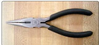
Figure 6-44. Needle-nose pliers.
