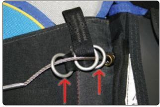
Figure 2-55. Double-ring container installation.
