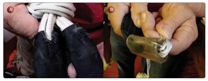
Figure 7-4. Protector damage.
