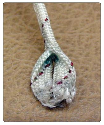
Figure 5-18. Worn closing loop.
