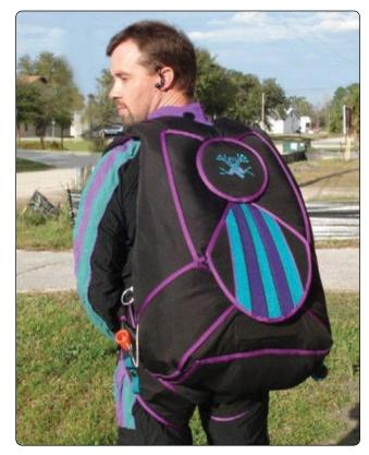
Figure 2-9. Tandem container system.
