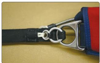
Figure 4-47. 3-ring assembled (from front).
