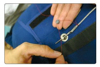
Figure 5-66. Threading the seal thread.
