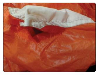
Figure 7-11. Pilot chute attachment damage is not always obvious.
