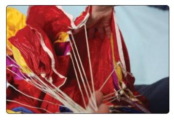
**Figure 4-10.** Separate and clear the material between the line groups.
