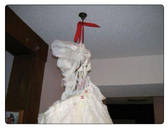
**Figure 6-89.** A square canopy can also be aired by S folding and hanging it from a simple hook.
