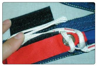
Figure 5-84. Set the deployment brakes.
