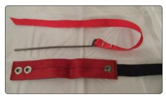
Figure 6-24. Pilot chute rod and strap.
