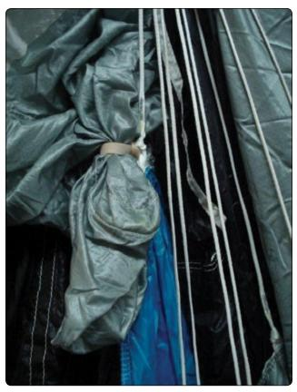
**Figure 4-37.** *Rubber band on center C-Line attachment tab holding apex of slider.*
