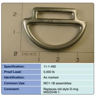
Figure 3-56. "D" ring harness, new style.
