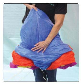
Figure 4-15. *Press the air out of the canopy.*
