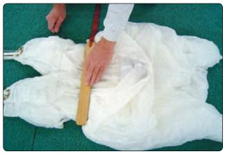
Figure 5-91. Packing paddle at <sup>1</sup>/<sub>3</sub>rd location.
