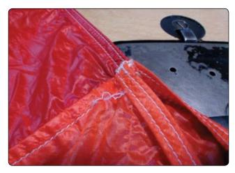
Figure 7-8. End seam damage.
