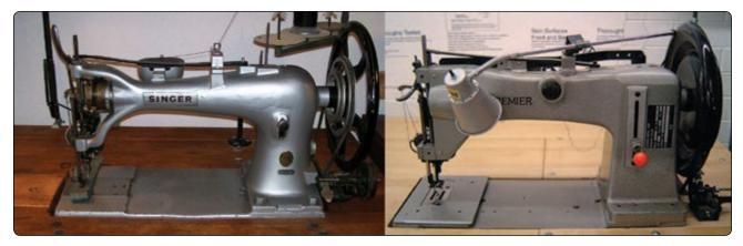
Figure 6-64. On the left is a Singer 7-34 heavy duty harness sewing machine and on the right is a Consew 733R.
