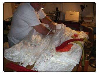
**Figure 6-87.** A square canopy being packed on a table, which must be accessible from both sides of the table in order to inspect and fold it properly.
