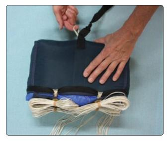
Figure 4-33. Pull pilot chute kill line from bottom of bag.
