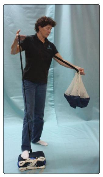
Figure 4-34. Pull the kill line through the bridle.
