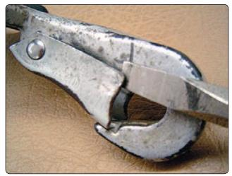
Figure 5-16. B-12 snap gate repair.
