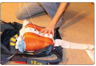
Figure 5-146. The bottom bodkin shown in place.
