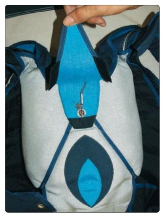
Figure 5-113. Close flap #4 and insert ripcord pin.
