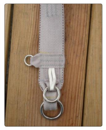
Figure 2-53. Main riser RSL ring attachment.
