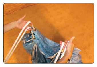
Figure 5-117. Push the slider up to the slider stops.
