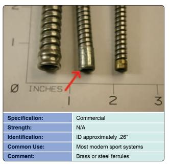
Figure 3-96. Housing, flexible, ripcord.
