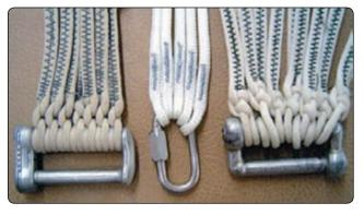
Figure 5-14. Three types of connector links.
