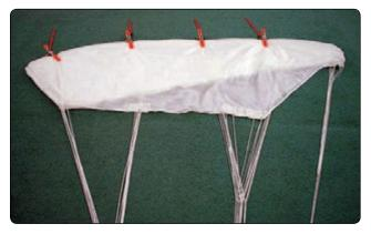
Figure 5-73. Clamps on top of canopy.
