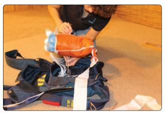
**Figure 5-145.** A bodkin that has been pre-loaded through the backpad of the container can now be easily pulled through the bag using this second bodkin.
