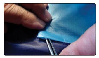
Figure 7-20. Confirming patch alignment.
