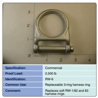
Figure 3-76. Ring, harness, replaceable, 3-ring.
