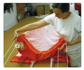
Figure 5-8. Round canopy—four-line check at canopy.
