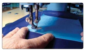
Figure 7-18. Start patch to damage.
