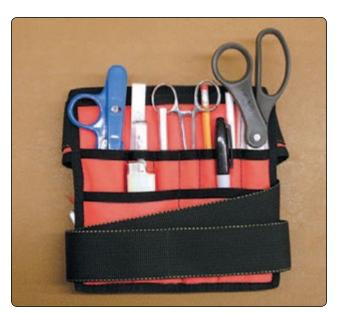
Figure 6-3. Rigger's tool belt.
