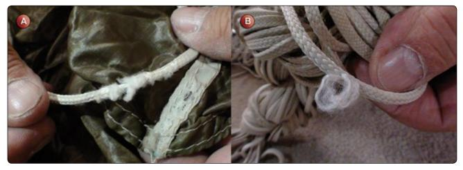
Figure 7-5. Line damage.
