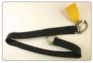
Figure 2-57. One style of RSL lanyard without Velcro.
