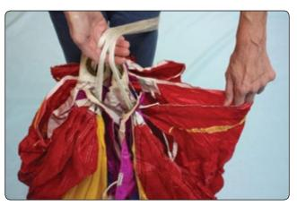
**Figure 4-9.** *Flake the canopy fabric between the* A-B, B-C, C-D *line groups following the perimeter of the canopy.*
