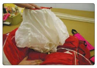
Figure 4-55. *Type 1 deployment in a pilot emergency rig.*
