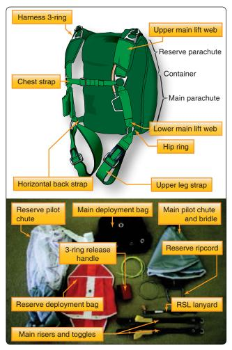
Figure 2-2. *Subcomponents of the harness/container assembly.*
