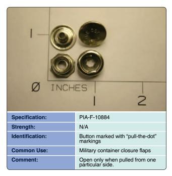
Figure 3-92. DOT Fasteners, Pull-the-dot.
