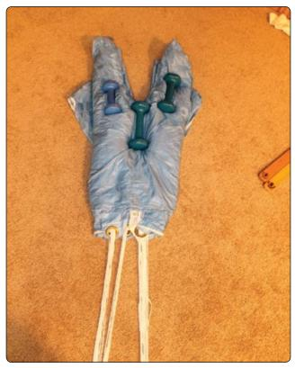
**Figure 5-130.** *Accordion the center cell, dividing the canopy in half. Weights can be used to control the pack job.*
