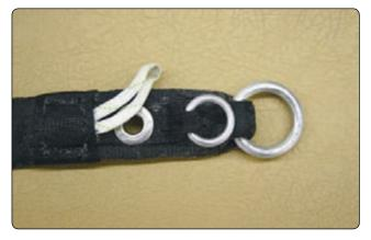
Figure 4-49. Riser release end.
