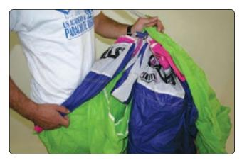
Figure 4-36. Rolling the nose of the canopy.
