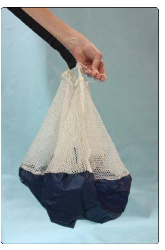
Figure 4-35. Drop the excess line into the pilotchute.
