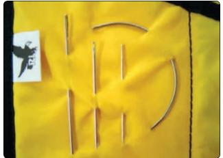
Figure 6-34. Hand tacking needles.
