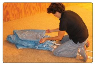
**Figure 5-128.** *Without disturbing the rest of the folds, pull the center tail section down to the slider grommets.*
