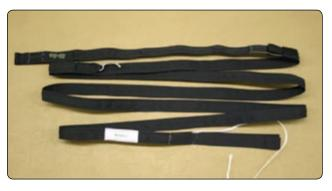
Figure 2-37. Kill-line collapsible bridle.
