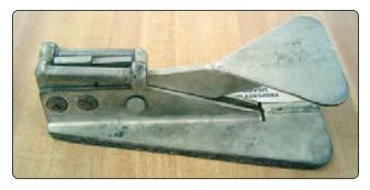
Figure 6-26. Connector link separator tool.
