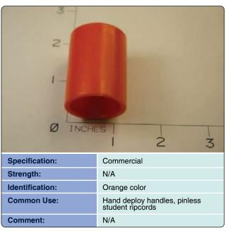
Figure 3-87. *HDPE tubing*, 1 <sup>1</sup>/<sub>2</sub>".
