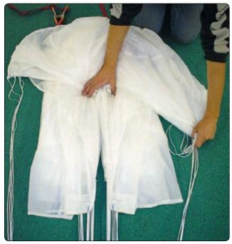
Figure 5-83. Pull down the trailing edge.
