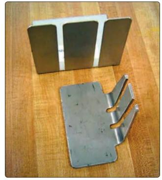
Figure 6-25. *Line separator (suspension line holder).*
