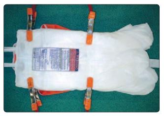
Figure 5-95. Bag positioned under canopy.
