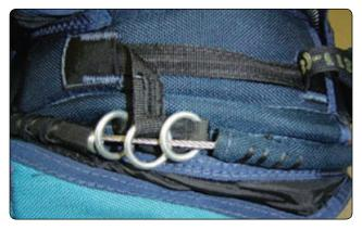
Figure 2-58. Ripcord cable routing through rings.
