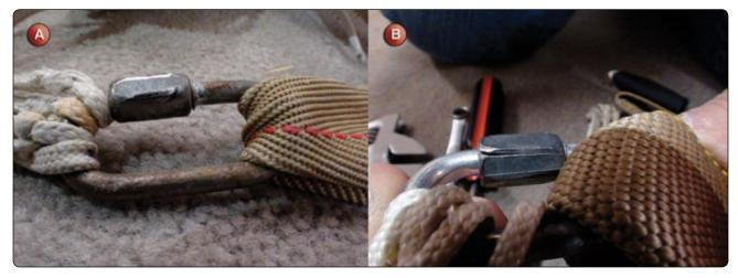
Figure 7-2. Link damage.
