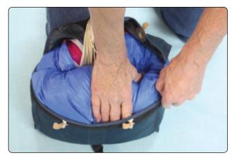
Figure 4-27. Shove the canopy down into the bag filling the corners.
