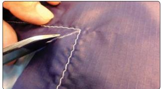
Figure 7-24. Corner seam cut.
