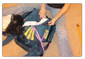
**Figure 5-153.** Insert bodkin through the top grommets of the backpad and bag and close upper side flap. There should be little or no canopy fabric in this upper area if good division of the ears has been maintained.
