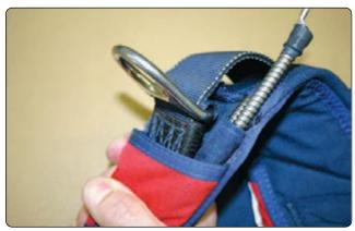
Figure 4-48. Harness 3-ring inspection.
