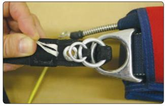
Figure 4-42. 3-ring small through middle ring.
