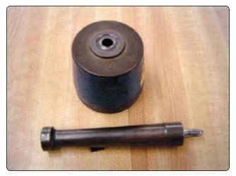
Figure 6-52. Size "O" rolled rim spur grommet handset.
