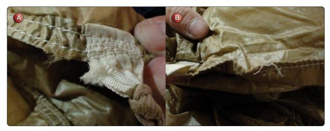
Figure 7-7. Line attachment damage.
