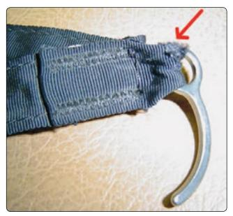
Figure 5-28. TOP bridle with worn pin tape.
