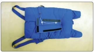
Figure 5-63. Ripcord pins in place.
