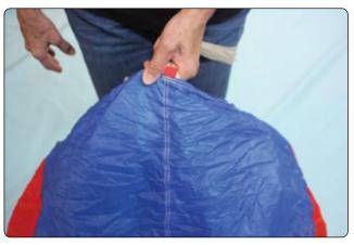
**Figure 4-13.** *Pull the tail up over the canopy and hold it under your thumb.*
