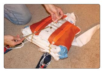
**Figure 5-143.** *Pull a second bodkin through the bag using a pull up cord.*
