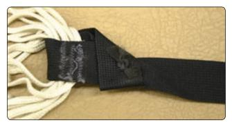
Figure 2-34. *Hand tack floating bridle loop.*
