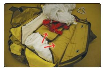
Figure 4-56. *Type 1 deployment in a sport piggyback.*
