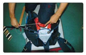
Figure 5-109. Position pilot chute.
