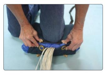
**Figure 4-29.** The closing flap of the bag is pulled so that the grommets meet the rubber bands. You should not have to stretch the rubber bands very far.
