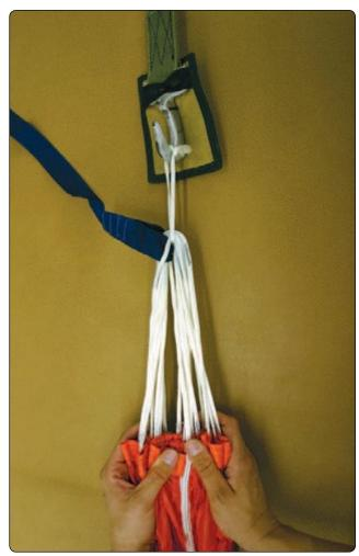
Figure 5-34. *Straightening the canopy apex.*
