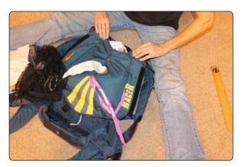
**Figure 5-154.** *Close other side flap leaving a short section of bridle below the pilot chute.*
