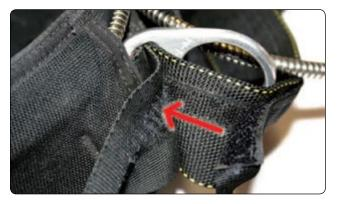
Figure 2-56. RSL Velcro riser damage.
