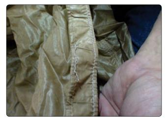
Figure 7-9. Long seam damage.
