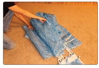
**Figure 5-124.** *If the PRO packed canopy was laid down carefully, it will be essentially flaked. Only minor straightening is necessary.*
