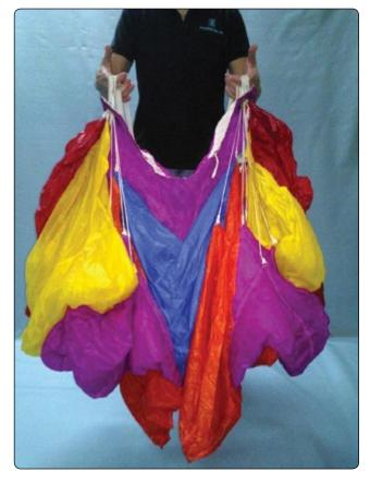
**Figure 4-6.** *The nose of the canopy is facing the packer. The tail of the canopy is facing outward.*
