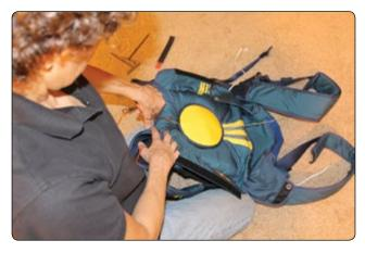
**Figure 5-164.** *Insert running ends into the isolated space between pilot chute "Hat" and top of the spring, using a hemostat or tweezers.*
