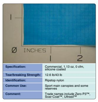
Figure 3-4. Cloth, parachute, nylon, Type-1, zero porosity.
