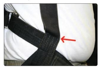
**Figure 2-18.** *Stair-stepped harness (aka stepped harness) junction warping.*
