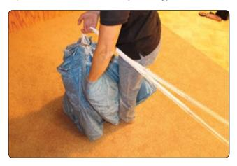
**Figure 5-119.** *Hold all flaked nose cells between the knees. Reach down and flake out material between A/B, B/C, and C/D lines.*
