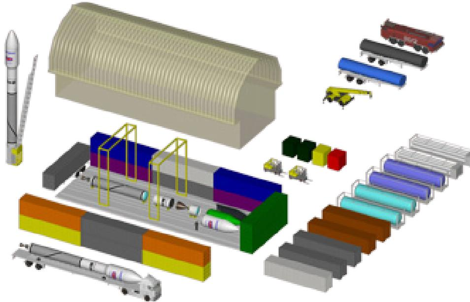
*The Black Arrow 2 launch facility is unique in that it is designed to be transported to various launch sites depending on customer needs. All the facilities can be stowed in 26 standard ISO cargo-containers and can be relocated to a new launch site in less than 30 days. (Source: Horizon Space Technologies)*
