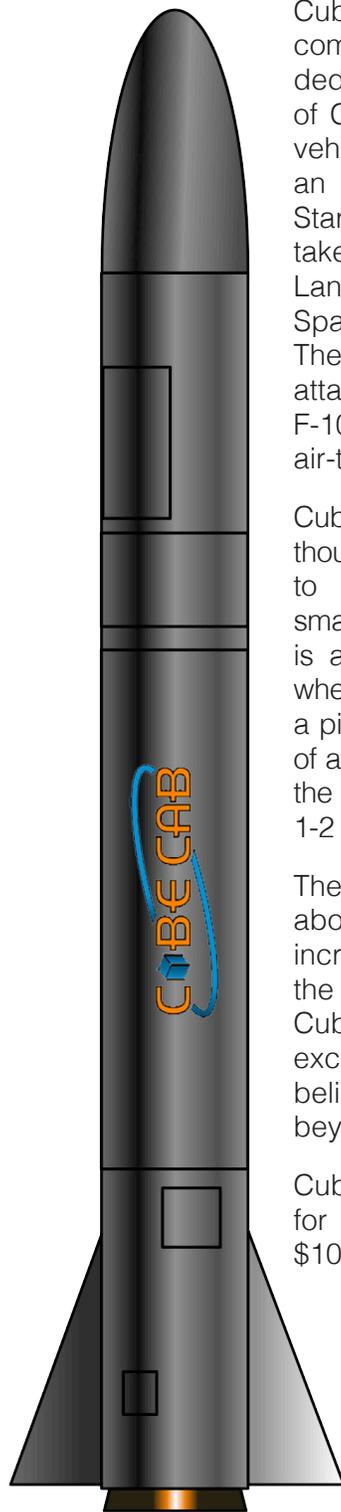
CubeCab is a U.S.-based company seeking to provide dedicated launches for operators of CubeSats. The relatively small vehicle will be launched from an F-104 Starfighter offered by Starfighters Aerospace that will take off from NASA's Shuttle Landing Facility at Kennedy Space Center (KSC) in Florida. The CubeCab vehicle will be attached below the wing of the F-104 in a similar manner to an air-to-air missile.
