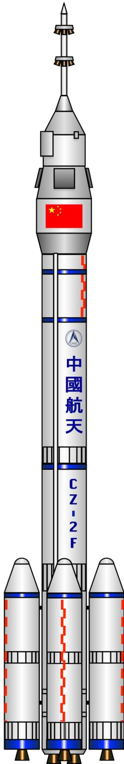
The Long March 2F, introduced in 1999, is China's only vehicle designed to transport astronauts. The two-stage vehicle is ultimately derived from the Long March 2C via the Long March 2E, a retired vehicle that was used to send payloads to geosynchronous orbit (GEO).
