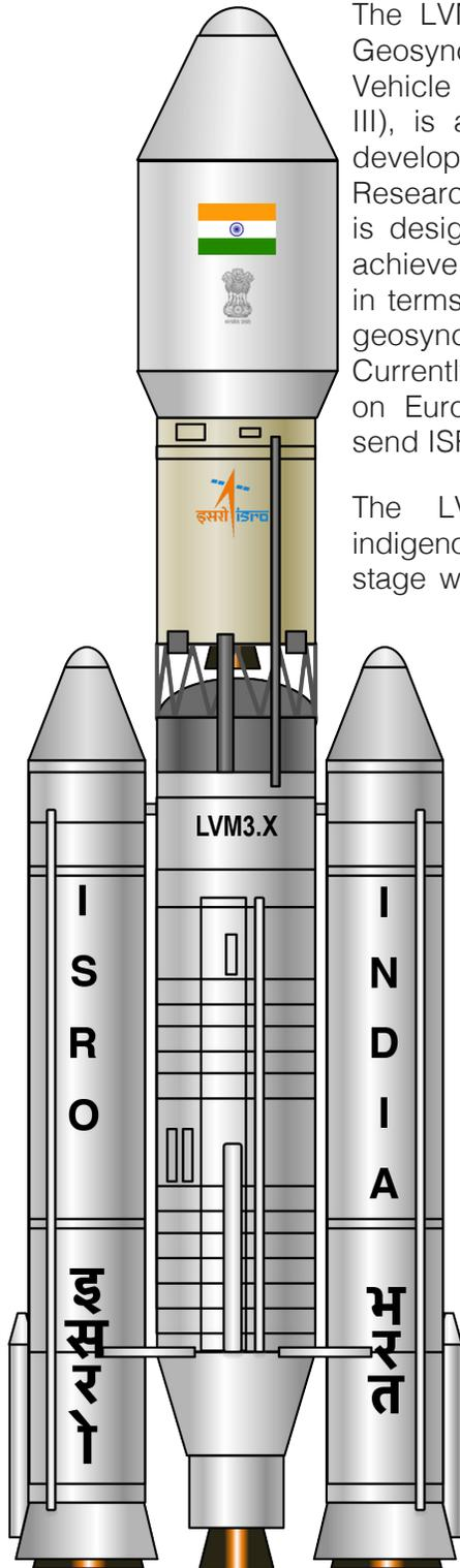
The LVM3, formally called the Geosynchronous Space Launch Vehicle Mark III (GSLV Mk III), is a launch vehicle being developed by the Indian Space Research organization (ISRO). It is designed to enable India to achieve complete self reliance in terms of sending satellites to geosynchronous orbits (GEO). Currently, India largely depends on Europe's Ariane 5 ECA to send ISRO payloads to GEO.
