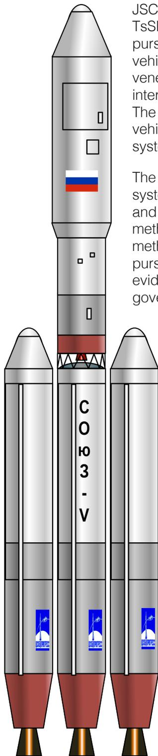
JSC SRC Progress (formerly TsSKB Progress) is currently pursuing the Soyuz 5, a family of vehicles designed to replace the venerable R-7 derived from the R-7 intercontinental ballistic missile. The Soyuz 5 is an entirely different vehicle, being a wholly new vehicle system.
