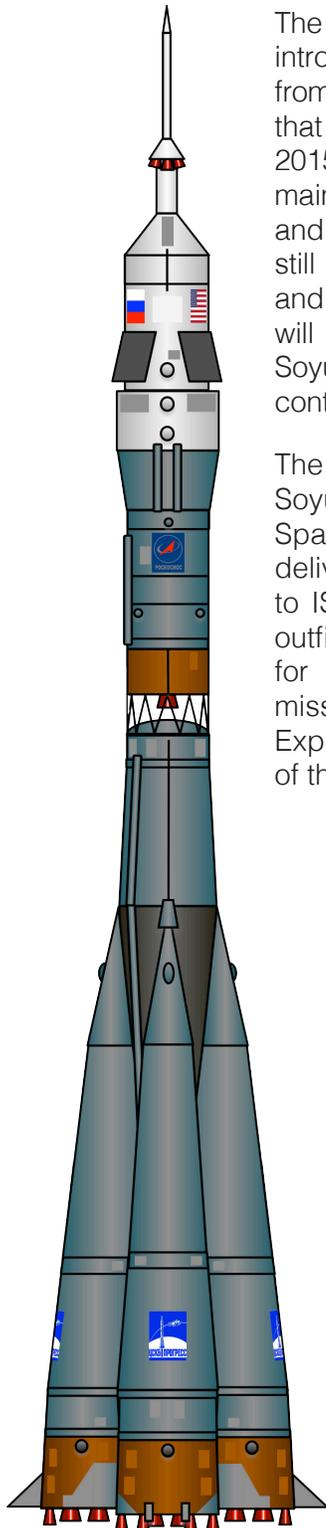
The Soyuz FG vehicle (11A511FG), introduced in 2001, is an improvement from the Soyuz U (11A511U) vehicle that was in service from 1973 to 2015. The improvements focused mainly on upgrades to the RD-108 and RD-107 engines. The vehicle still uses an analog control system, and it is anticipated that the vehicle will ultimately be replaced by the Soyuz 2 series, which has a digital control system.
