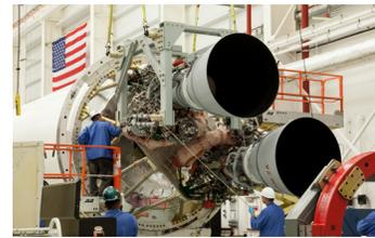
Two RD-181 beng integrated with an Antares launch vehicle (NASA)
