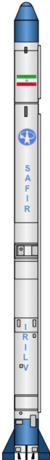
Iran's Safir launch vehicle is based on the Shahab 3 ballistic missile. The Shahab 3, based on the North Korean Nodong-1 ballistic missile, was in service from 1998 through 2003. Though the Safir may have been launched during an attempt in 2007 (there is confusion on what vehicle was used during the flight test), the first confirmed launch of Safir occurred in 2008. This suborbital flight was followed by six orbital launch attempts, four of which have been considered successful.
