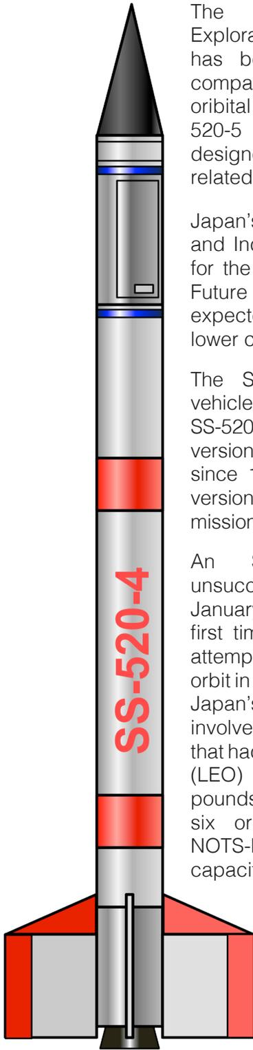
The Japan Aerospace and Exploration Agency (JAXA) has been working with several companies to develop a very small orbital launch vehicle. The SS-520-5 is a development vehicle designed to gather data for use in related future programs.
