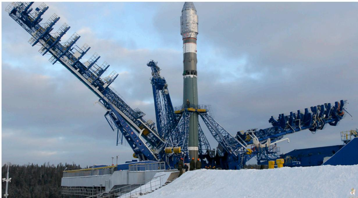
A Soyuz 2.1v is prepared for launch in December 2015. The launch, carrying a Kanopus remote sensing satellite, did not go entirely as planned - the payload did not fully separate from the upper stage due to a second stage latching problem. (Source: Russian MoD)
