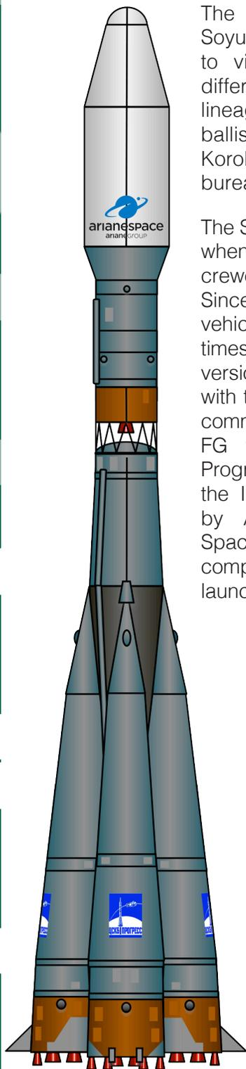
The Soyuz 2 (also referred to as Soyuz ST) is used to launch satellites to virtually any orbit from three different launch sites. It can trace its lineage to the R-7 intercontinental ballistic missile designed by Sergei Korolov and his OKB-1 design bureau in the mid-1950s.
