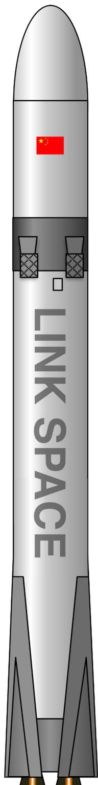
China-based Link Space, founded in 2014, is developing a two-stage, small orbital launch vehicle called New Line 1 (Xin Gan Xian 1) with a reusable first stage. The vehicle is based on a successfully tested suborbital rocket called KC-SA-TOP.
