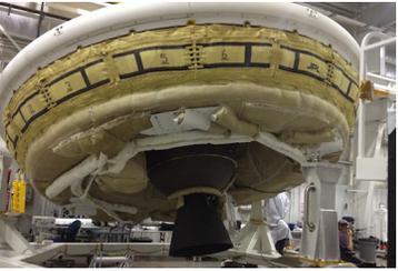
*A STAR-48 motor used for NASA's Low-Density Supersonic Decelerator project (NASA)*
