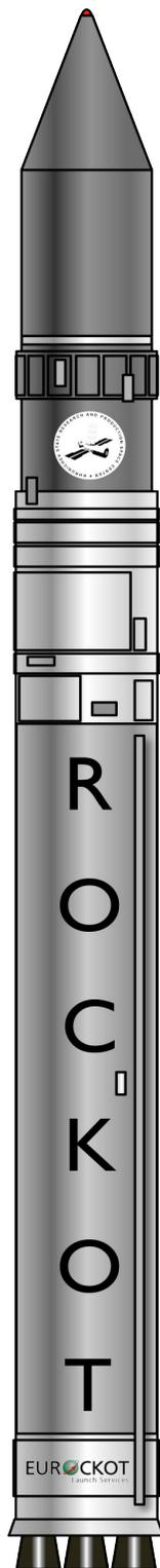
The three-stage Rocket is developed using refurbished missile components. The missile used as the basis for the commercially available vehicle is the UR100N (SS-19) intercontinental ballistic missile (ICBM) built by Soviet-era OKB-52. Production and launch of the Rocket is managed by Eurockot Launch Services GmbH, a joint company between Russia's Khrunichev State Research and Production Space Center and EADS Astrium.
