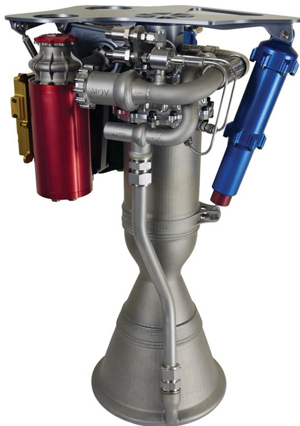
Rocket Lab's Rutherford engine. All its primary components are produced using additive manufacturing, or 3D printing. (Source: Rocket Lab)
