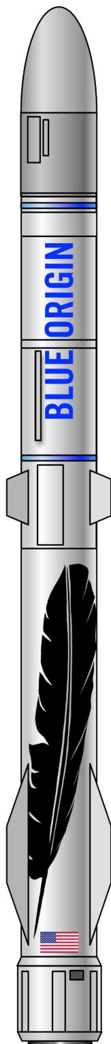
In the summer of 2015, Blue Origin publicly announced its plan to develop an orbital launch vehicle. Details regarding the vehicle's design remained close-hold until 2016, when the company introduced its New Glenn family of vehicles. The New Glenn family will feature a reusable first stage with six landing struts, and will burn liquid oxygen (LOX) and liquified natural gas (LNG). The tanks will be pressurized without helium, a rare characteristic for launch vehicles employing liquid propellants.
