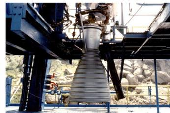
An RS-27A undergoing ground testing (Aerojet Rocketdyne)
