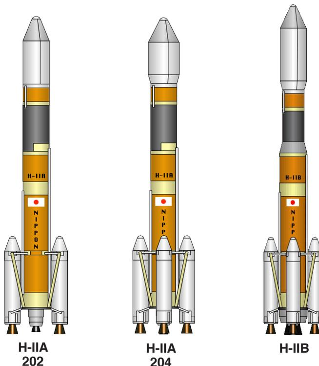
The H-IIA is used for a variety of missions and represents the workhorse launch vehicle for Japan. The H-IIB has been used exclusively to send cargo to the ISS, but recently MHI Launch Services has made the vehicle available for commercial use.
