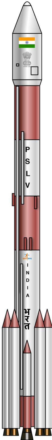
The Indian Space Research Organization (ISRO) has offered the Polar Satellite Launch Vehicle (PSLV) since 1993. The vehicle is used to launch small and medium payloads to low Earth orbit and, on occasion, to send small satellites to geosynchronous orbit. For missions to LEO, it is not uncommon for the PSLV to launch several satellites at a time.
