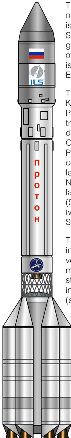
The Proton Medium, a 2-stage version of the venerable Proton M vehicle, is provided by International Launch Services (ILS) as a launch option for government and commercial operators of satellites in geosynchronous orbit. It is typically not used for missions to low Earth orbit (LEO).
