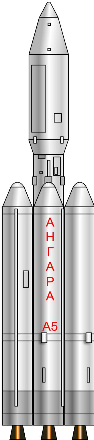
The Khrunichev State Research and Production Space Center has been developing the Angara series of vehicles to replace virtually all vehicles in service with the exception of the Soyuz. The Angara 1.2 is expected to replace the Rockot and Dnepr while the Angara A5 is expected to replace the Proton M within 5-7 years. The Universal Rocket Module (URM-1) forms the modular core of every Angara vehicle, with a URM-2 used as a second stage. A Breeze-M upper stage serves as an optional third stage.
