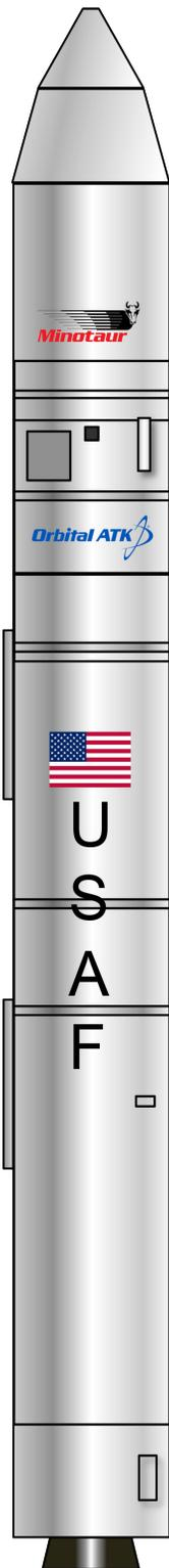
The Minotaur IV is an orbital launch vehicle offered by Orbital ATK. The vehicle is derived from the Peacekeeper intercontinental ballistic missile (ICBM).
