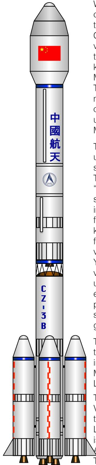
With a low Earth orbit (LEO) capacity of 12,000 kg (26,456 lb), the Long March 3B is currently China's most powerful launch vehicle. The vehicle is derived from the Long March 3A vehicle, with the key difference being that the Long March 3B uses four liquid boosters. The vehicle is primarily used for missions to a geostationary transfer orbit (GTO), but can be used for uncrewed science missions to the Moon (Chang'e-3).
