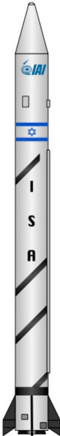
The Shavit 2 is an orbital launch vehicle developed by Israel. The Shavit 1, launched for the first time in 1988, was based on the Jericho II missile. The more powerful Shavit 2 vehicle was introduced in 2007 and is the current version being used.
