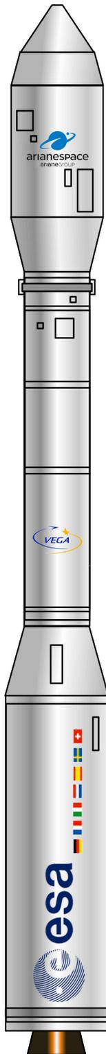
The Vega launch vehicle, named after the second brightest star in the northern hemisphere, is operated by Arianespace and targets payloads to polar and low Earth orbits used by scientific and Earth observation satellites. It is manufactured by ELV SpA, a joint venture between Italy-based Avio SpA and the Italian Space Agency (ISA).
