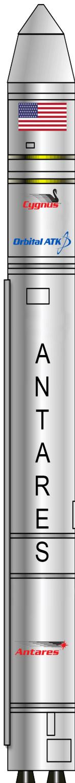
In 2013, Orbital Sciences Corporation (now Orbital ATK) began offering its Antares, a two-stage vehicle designed to launch government and commercial satellites to low Earth orbit (LEO), Cygnus cargo modules to the International Space Station (ISS), and missions requiring Earth escape trajectories. The Antares is also available under the NASA Launch Services (NLS) II contract for future science missions.
