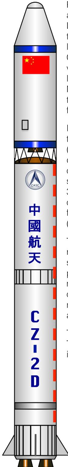
Primarily used to lift payloads to LEO and SSO, the 41-meter-tall, two-stage Long March 2D launch vehicle is part of the Long March 2 family of rockets. First launched from Jiuquan Satellite Launch Center in 1992, this Chinese launch vehicle has completed 25 successful launches. Two variants of the Long March 2D are known, and both are two-stage rockets that employ engines fueled by  $N_2O_4$ /UDMH.
