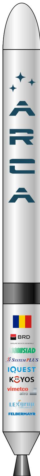
Developed by the Aeronautics and Cosmonautics Romanian Association (ARCA) as part of its bid to win the Google Lunar X Prize, the Haas 2C is a 2-stage orbital launch vehicle. The vehicle is named after Transylvanian Conrad Haas, an engineer that explored staged rockets during the 16<sup>th</sup> century, well before Konstantin Tsiolkovsky published his rocket equation in 1903. In addition to rocket technology, ARCA develops aeronautical and ground transportation systems.
