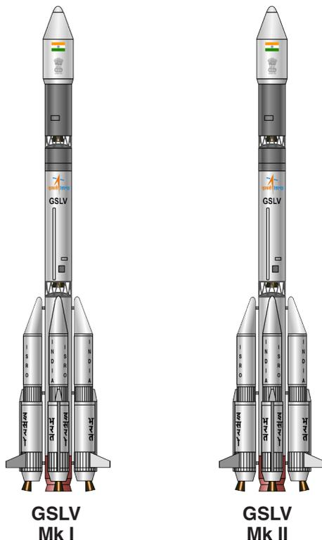
The GSLV Mk I has flown six times, while the GSLV Mk II has flown three times. There were three variants of the GSLV Mk I, each distinguished by differences in propellant capacity and quality across stages and solid boosters. Only one variant, the GSLV Mk I(c) remains in service. The GSLV Mk II differs from the Mk I primarily because of the third stage, which is built by ISRO. Upper stages used for the Mk I were built in Russia.
