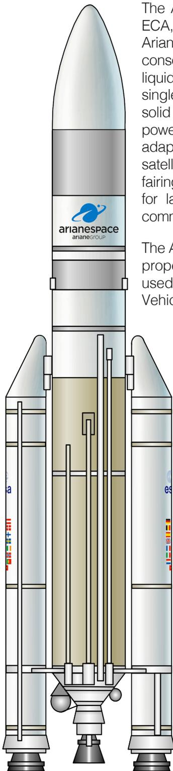
The Ariane 5, technically the Ariane 5 ECA, is the workhorse of France-based Arianespace, a European launch consortium. The Ariane 5 consists of a liquid-fueled core stage powered by a single Vulcain 2 engine, two strap-on solid boosters, a cryogenic upper stage powered by an HM7B engine, a payload adapter that can accommodate two satellites (called SYLDA), and a payload fairing. The Ariane 5 ECA is optimized for launches of two geosynchronous communications satellites.
