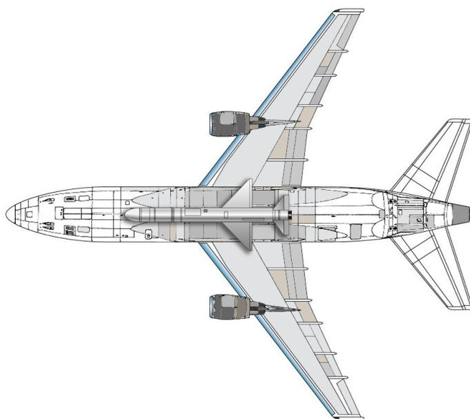
*Orbital ATK uses a modified L-1011 aircraft to carry and launch the Pegasus XL vehicle. The ground equipment necessary to launch the system is minimal, and the combination can be launched from almost any conventional runway.*
