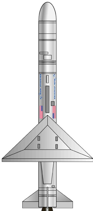
Orbital ATK's Pegasus XL is a small-class, air-launched vehicle. Orbital ATK offers the Pegasus XL as a means to launch small satellites to low Earth orbits (LEO).
