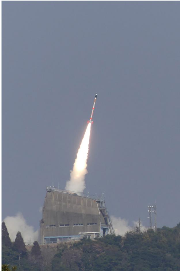
*The SS-520-5 is launched in January 2018 carrying a student-built CubeSat called TRICOM-1R. On this flight, the vehicle became the smallest ever to launch a payload into orbit. (Source: NVS)*
