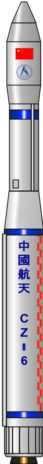
The Long March 6 is a cooperative effort between China Aerospace Science and Technology Corporation (CAST) and the China Academy of Launch Vehicle Technology (CALT). It is a small, liquid-fueled vehicle that has a low Earth orbit (LEO) payload capacity less than that provided by the currently available small-class Long March 2C, meaning the vehicle serves a niche previously not directly addressed.
