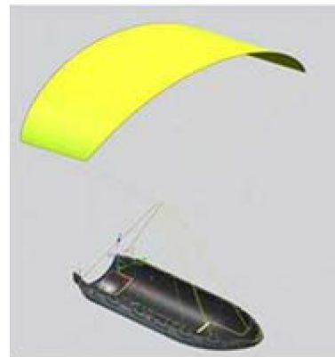
Figure 2. Payload fairing half with parafoil deployed
