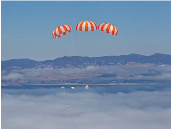
Figure 4. Dragon-1 Main Parachutes with (smaller) Drogue Parachutes (FAA 2017)
