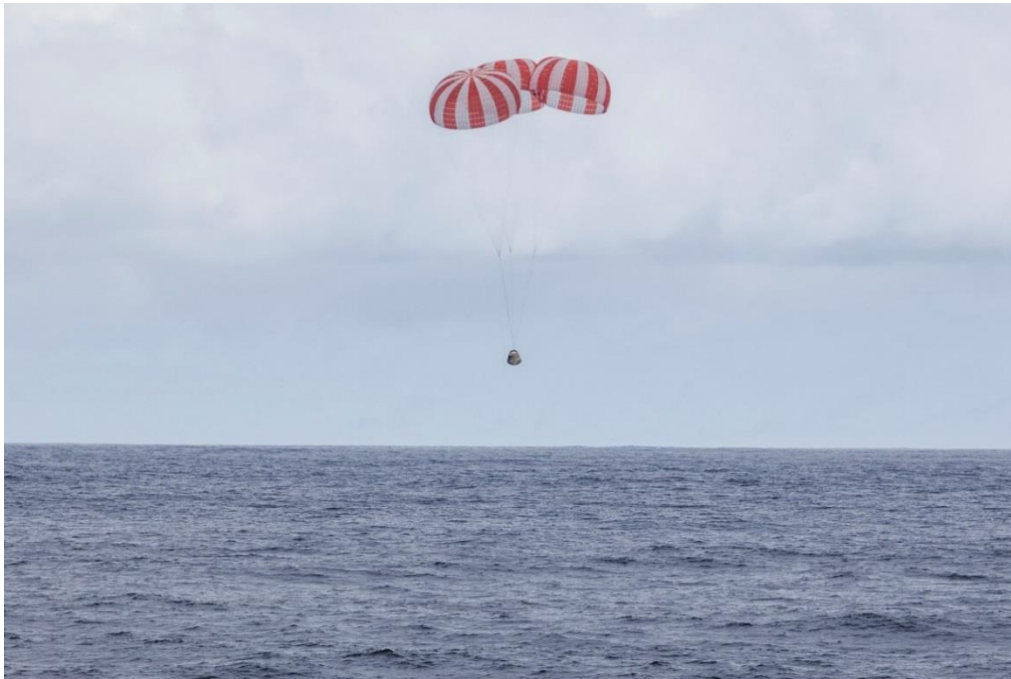
Exhibit 3. Dragon-1 Main Parachute Deployment
