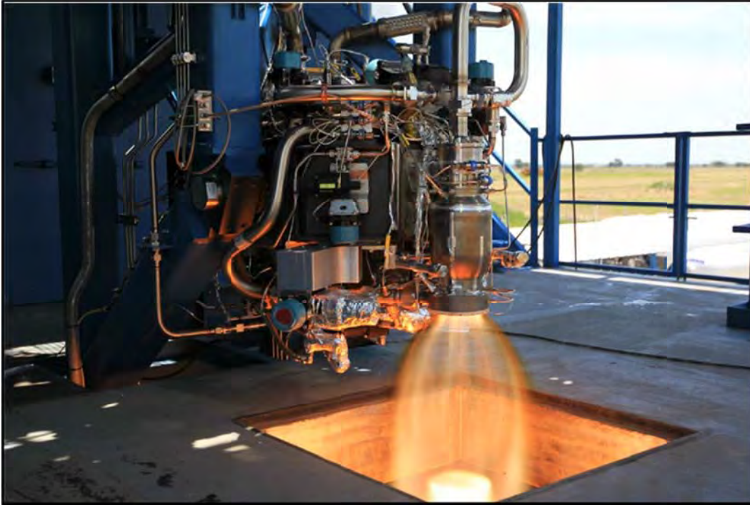
Figure 4. SuperDraco Engine at Full Throttle (Photo Courtesy of SpaceX)
