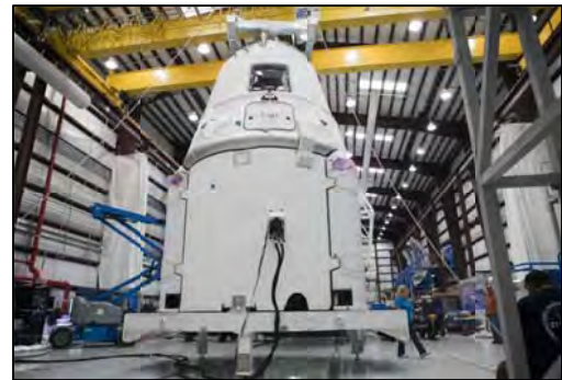
Dragon Capsule with Integrated Trunk
