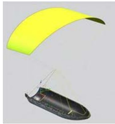
Figure 2. Payload fairing half with parafoil deployed
