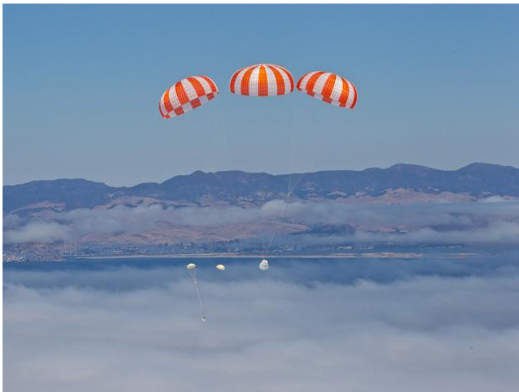
Exhibit 2. Dragon-1 Main Parachutes with Released Drogue Parachutes in the Background
