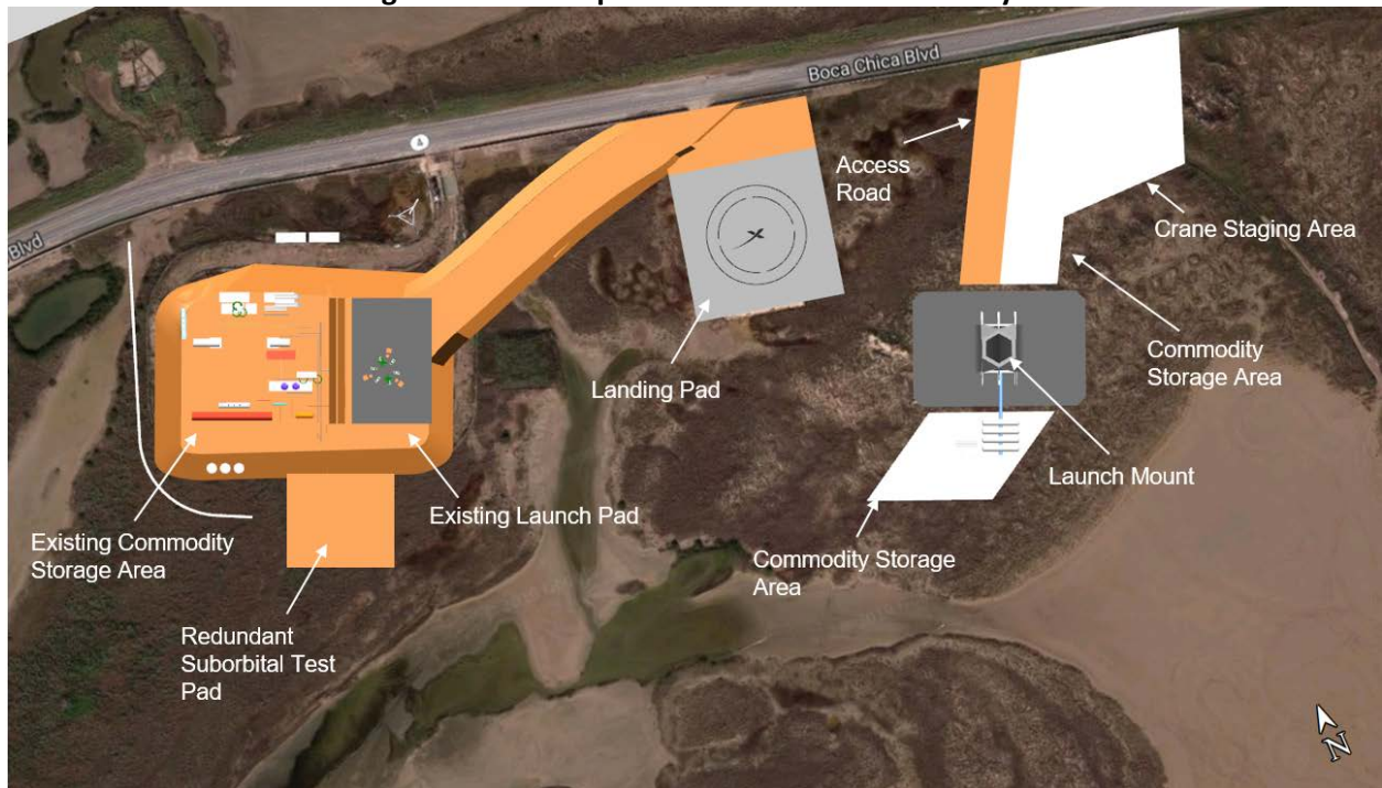
Figure 2. New Proposed Vertical Launch Area Layout
