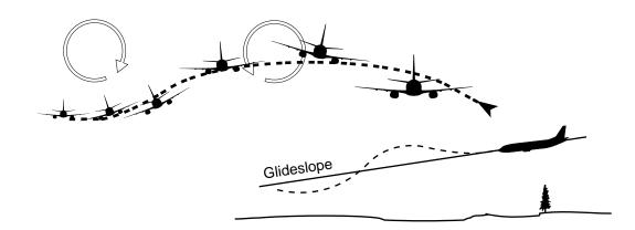
When approached from below, the downward flow through the wake pushes the aircraft down and away from the wake. If approached at a rapid enough rate, the aircraft will pass through the wake (See Figures 2.4-8 and 2.4-9).
