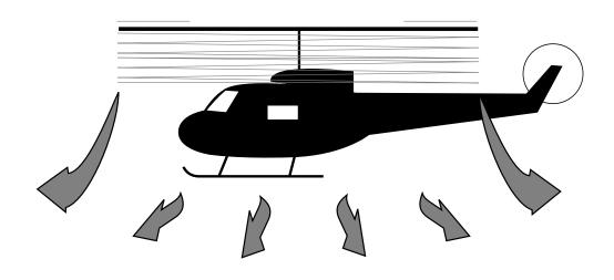
Figure 2.8-13 Helicopter hoverproduced downwash
