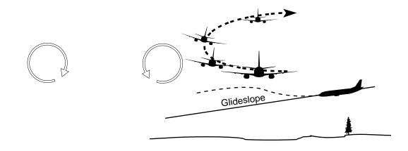
Figure 2.4-7 Aircraft reaction to wake turbulence encounter, rapid approach from the side (rear view depiction)
