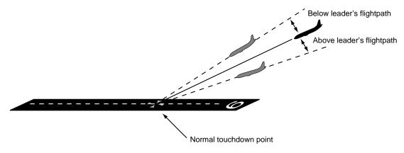
While following an aircraft, extending an imaginary line from your aircraft through the leader to the runway should end at the normal runway touchdown point (Figure 2.10-1B). If it ends at a point down the runway, the
