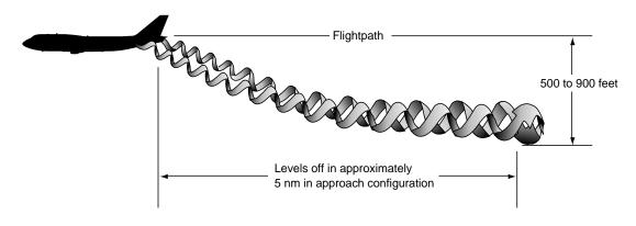
On approach and takeoff the wake descends below the flightpath until it enters ground effect whereupon the vortices slow their downward descent and move laterally as shown below. Typically, the wake's descent will be arrested within approximately 1/2 wingspan (50-100 feet for the B-747) of the ground. Be-
