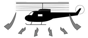
Figure 2.4-1B Formation of helicopter wake turbulence (forward flight)
