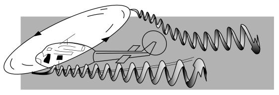
Figure 2.8-14 Helicopter forwardflight-produced wake turbulence
