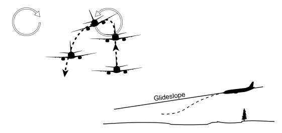
Figure 2.4-8 Aircraft reaction to wake-turbulence encounter, approach frome below right (rear view depiction)
