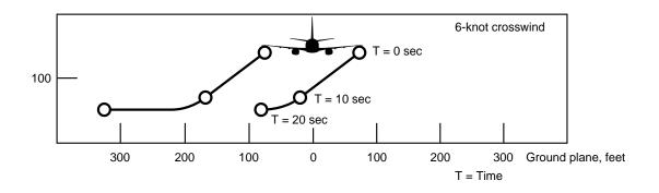
Vortices have been found to move laterally as much as 1500 feet under certain conditions, but with seemingly weak strengths at the larger lateral distances. Additionally, under some crosswind conditions, vortices have been observed to "bounce" (i.e., descend toward the ground and then later begin to rise up somewhat).
