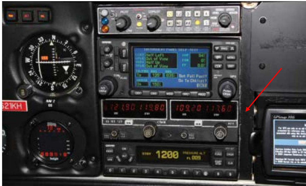
Figure 4. Aircraft Instrument Panel with VHF Communications Transceiver
