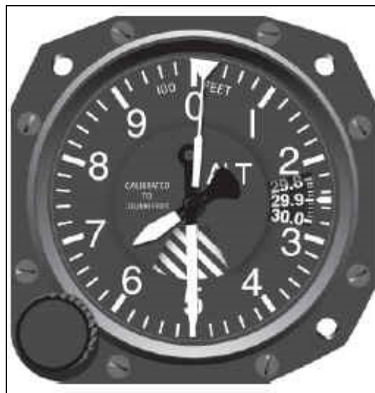
Figure 3-16. Dash-Mounted Pressure (or Barometric) Altimeter
