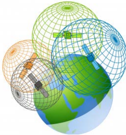
Figure 3-17. Satellite Based Trilateration
