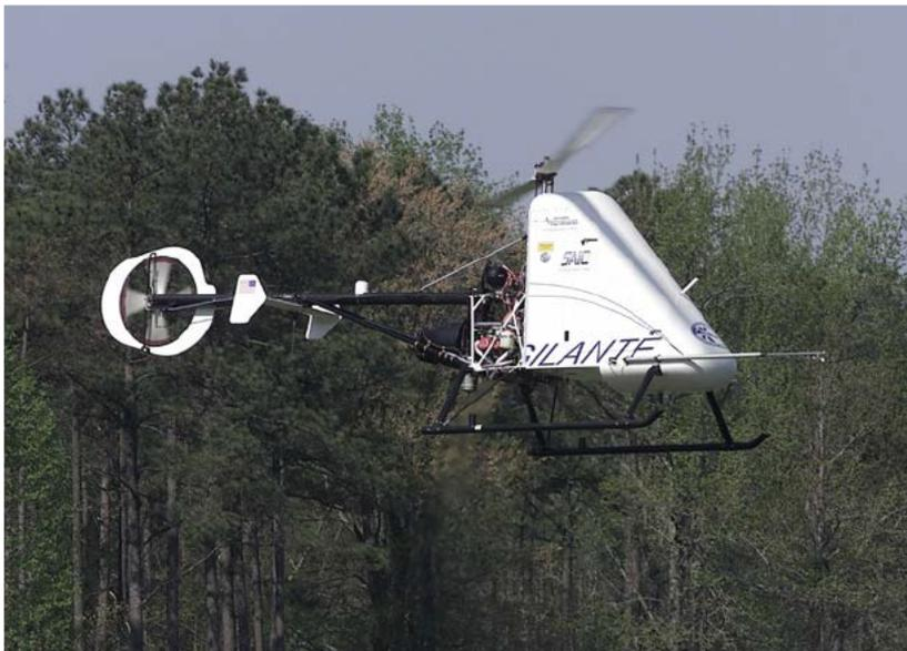
Vigilante serves as a testbed vehicle at AATD for testing and demonstrating manned-unmanned teaming and UAV technologies, including weapons and sensors.
