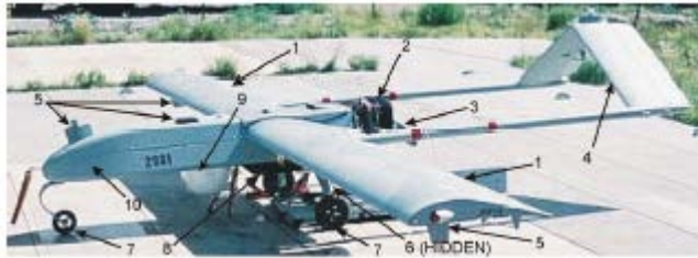
Figure 1. Shadow 200 TUAV, major hardware components.
