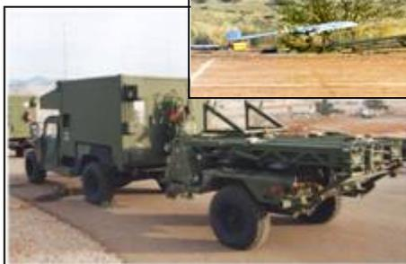
Air Vehicle Transport & Launcher Trailer
