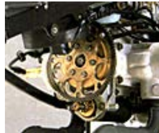
Fig 2-4. RMAX generator and engine flywheel.
