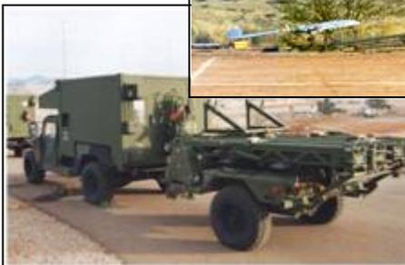
Air Vehicle Transport & Launcher Trailer
