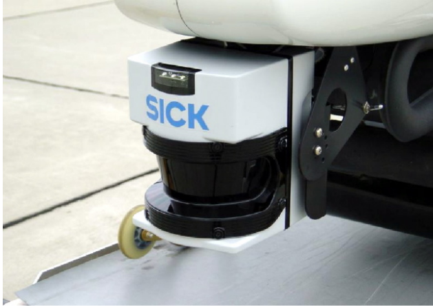
Figure 4. SICK LMS Class I (eye-safe) scanning laser rangefinder.
