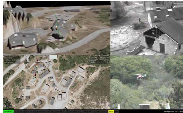
Fig 2-2. Screen capture of SA display in ARP ground station during autonomous landing; clockwise from lower right: ground station tracking camera, moving map display including planner messages, computer-generated view of helicopter driven by telemetry stream, live digital image stream from on-board camera, status and warning lights (bottom).
