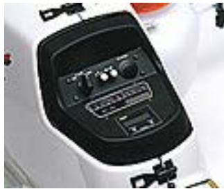
Fig 2-7. Back panel used for control mode selection.
