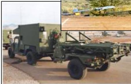
Air Vehicle Transport & Launcher Trailer
