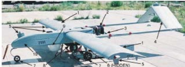
Figure 1. Shadow 200 TUAV, major hardware components.
