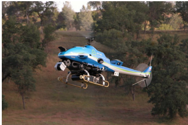
Fig 1-1. AFDD Autonomous Rotorcraft Project RMAX helicopter in operation at Fort Hunter Liggett in California.
