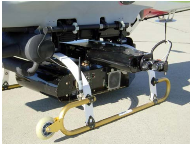
Figure 4-1. Avionics payload and stub wing.
