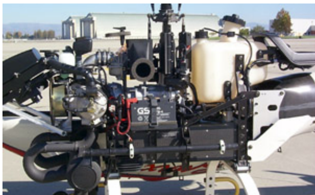
Fig 2-3. RMAX engine compartment.
