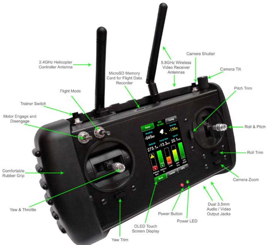
indicates transmitter battery health, aircraft battery health, data link quality, GPS satellites and quality of GPS.
