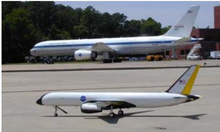
Figure 2-1: Typical AirSTAR Project UAS Scaled Pilot Trainer
