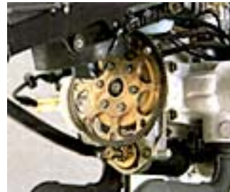
Fig 2-4. RMAX generator and engine flywheel.
