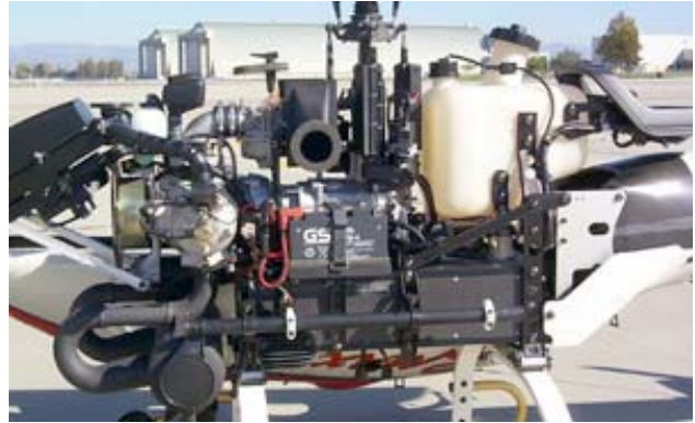
Fig 2-3. RMAX engine compartment.
