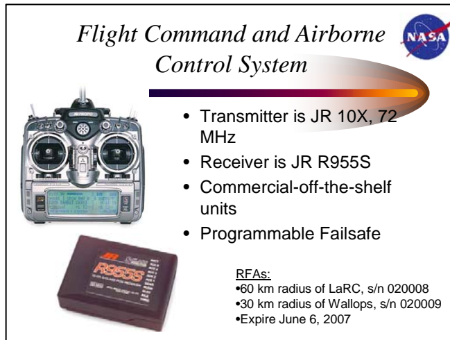
Figure 2-4: AirSTAR Project UAS Flight Command and Airborne Control System
