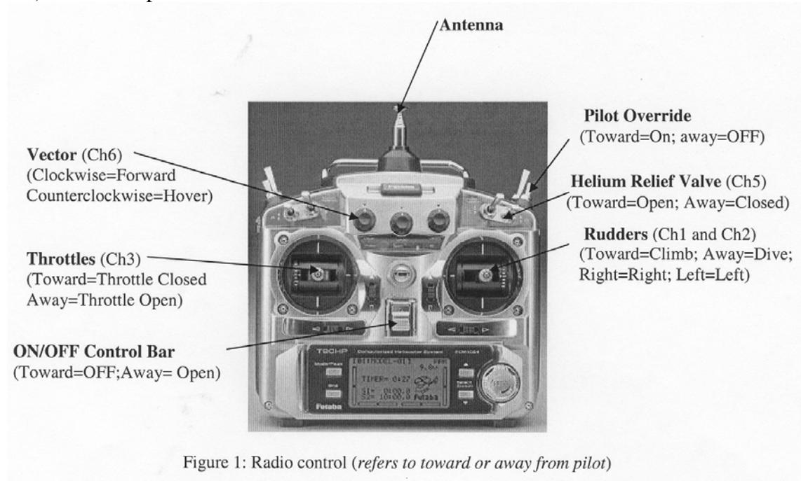
Figure 1: Radio control (refers to toward or away from pilot)
