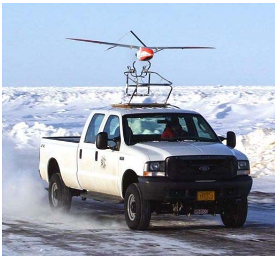
Aerosonde UAV rotating out of the rooftop cradle on launch
