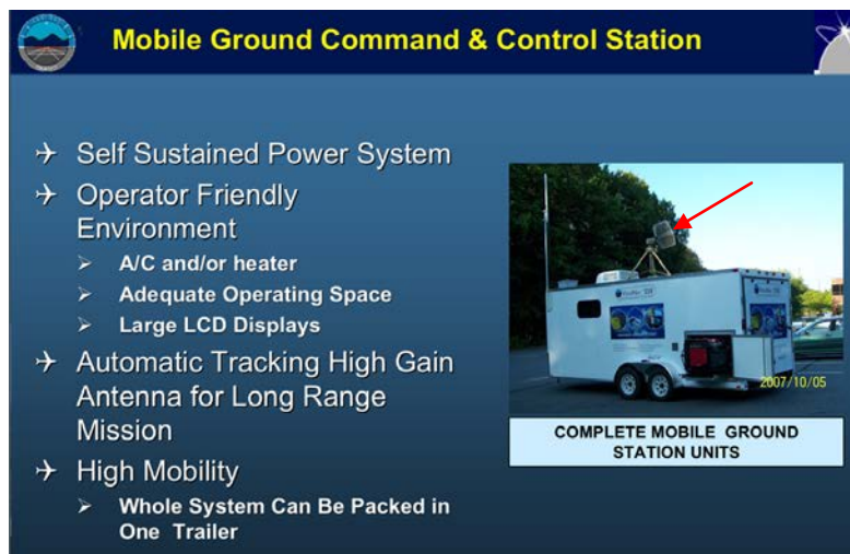
Figure 1. Vector-P mobile ground control station (GCS). Note tracking tripod assembly (see arrow) on roof, enabling line-of-sight command-and-control telemetry for longer range missions.
