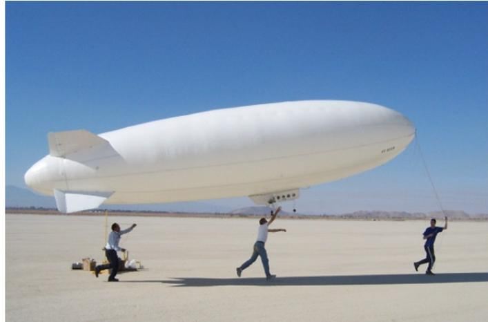
The blimp has two O.S. Max-108FSRring <BX-1> engines running on the typical RC model aircraft fuel containing 18% nitromethane. Teleoperation control is effected with a Futaba Model T9CP hand held control unit (pictured below) which operates over a standard 72 MHz link.
