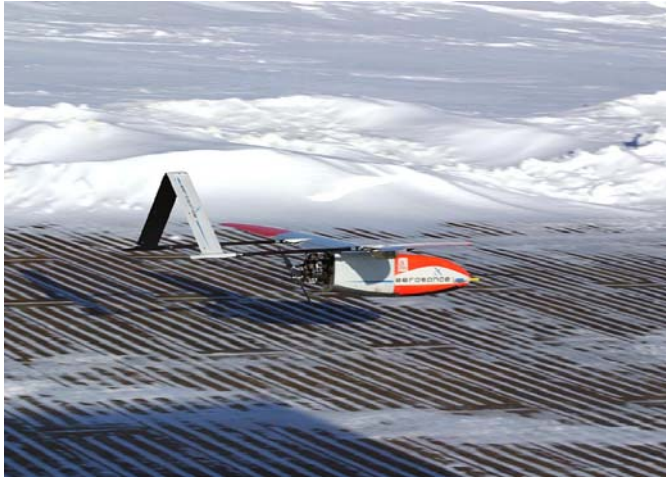
An Aerosonde air vehicle just before touchdown
