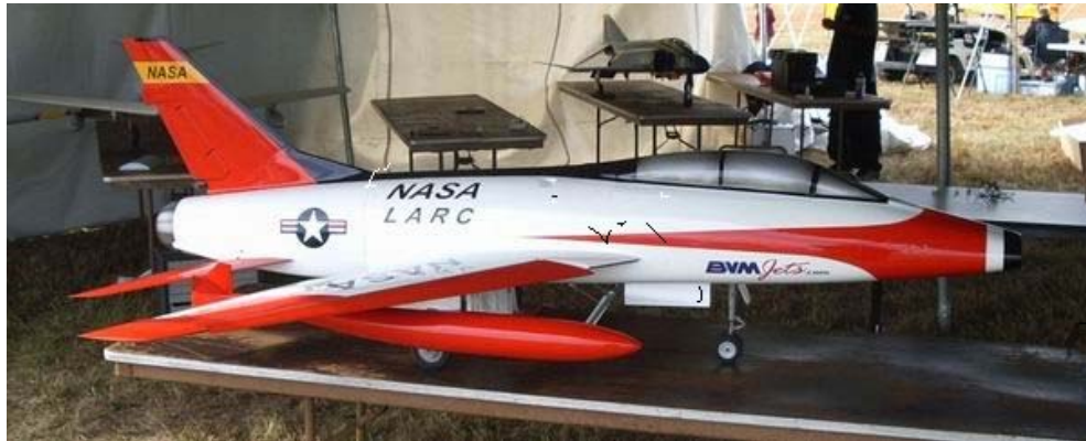
Fig. 2-1 F-100 AirSTAR Project UAS Scaled Pilot Trainer
