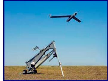
The launch sequence is fully automated. The Insight A-20 climbs on course until it reaches a pre-designated safe altitude, at which point it automatically turns to its next projected waypoint.
