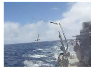
The entire approach and recovery process is fully automated. Thus, the aircraft is not placed at risk by the performance of an external pilot flying the plane in a manner similar to a remote control model, as is typically done with other UAS.
