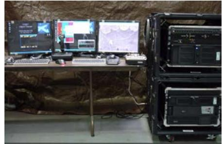
The control station consists of multiple (at-least two) MS-Windows based computer systems as well as a custom embedded controller. The MS-Windows flight software can be operated on both computers, allowing a high-degree of redundancy in the event of hardware failure in one of the MS-Windows computers.
