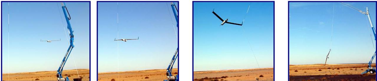
The entire approach and recovery process is fully automated. Thus, the aircraft is not placed at risk by the performance of an external pilot flying the plane in a manner similar to a remote control model, as is typically done with other UAS.
