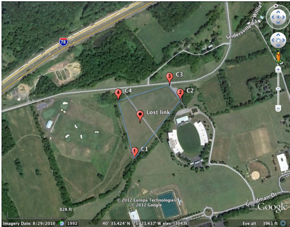
Figure 3: Detail view of UAV operations area. The blue outline shows the flight operations area. The lost link waypoint is labeled; take-off will occur by hand-launch in to the wind from the middle of the operations area.
