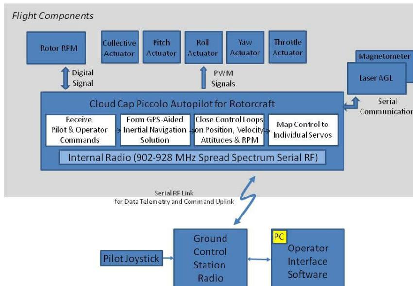
The autopilot for the flight test vehicles consists of the Cloud Cap Technology Avenger SL Autopilot. The commercial off-the-shelf Avenger autopilot system for rotorcraft provides fully automated flight operations, including take-off, waypoint following, and landing, and also modes
