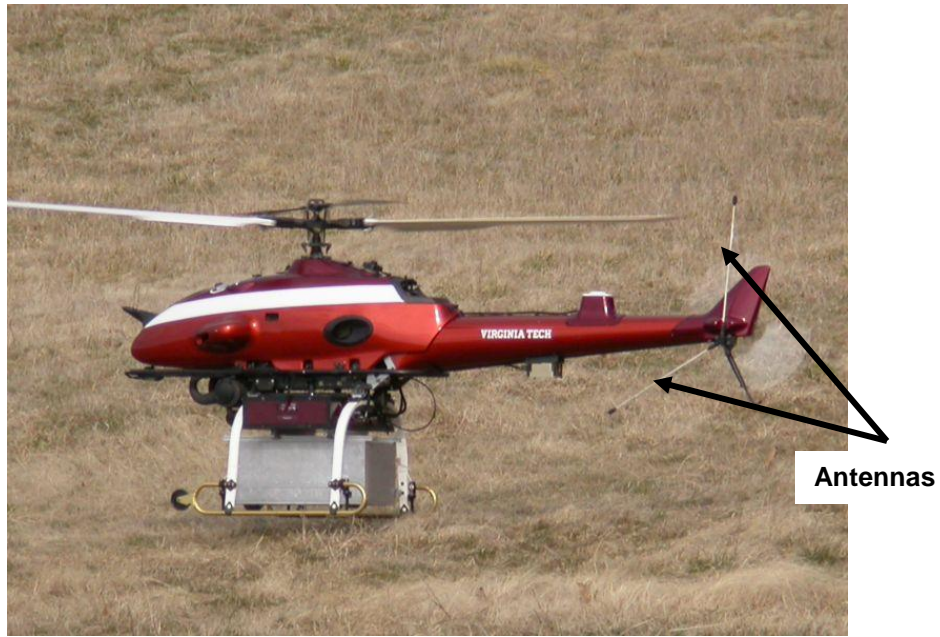
Figure 2 – RMAX antenna placement
