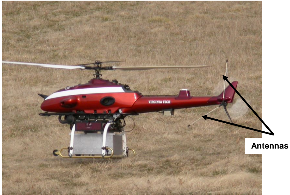
Figure 2 – RMAX antenna placement
