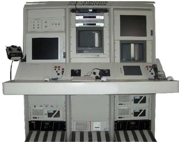
The LRS is a portable version of the GCS with a single position incorporating both IP and PO functions. It is primarily used when the GCS is not physically located at the launch and recovery site. This allows distributed operations where the Aerostar UA can be launched and then passed forward to the MCS located in the mission area for greater operating distances.
