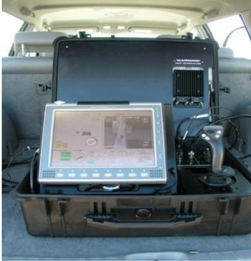
The Remote Payload Control Station (RPCS) provides control of the payload system and display from a location other than the GCS or LRS.
