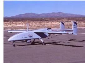
For the recovery process, flight control of the Aerostar UA is transferred from the IP to the EP pilot after the EP makes visual contact with the Aerostar UA and has informed the IP that he/she is ready to assume flight control of the Aerostar UA. Thereafter, the EP controls the Aerostar UA during the approach and landing. After landing the Aerostar is loaded on the transportation dolly and transported off of the runway/strip
