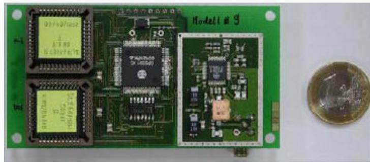
Figure 7. GPS Orion-HD receiver for sounding rocket tracking and IIP prediction [19]
