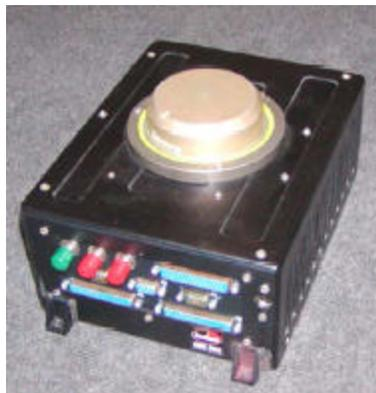
Figure 8. SpaceShip One’s System Navigation Unit [24]
