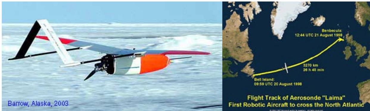
Figure 5. The Aerosonde UAV and its Flightpath across the Atlantic [42]
