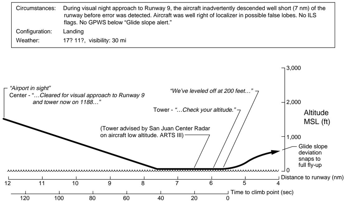
The GPWS never alerted the crew to the low glide slope because the ILS had locked on to a false lobe, and it had never alerted the flight crew to the altitude deviation because the gear was down and the flaps were in the landing position. The GPWS was operating normally, because it used inputs from the Captain's instruments that reflected an on-glide-slope condition. The GPWS never reached a limit that was considered out of tolerance.
