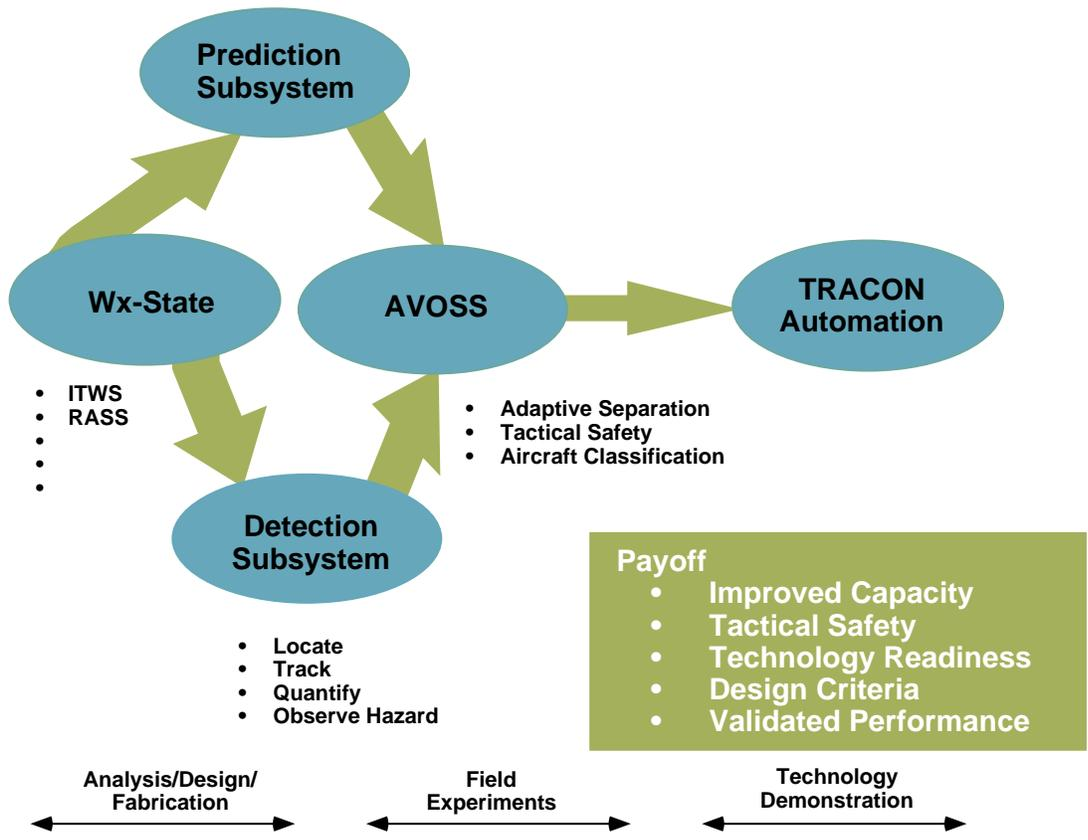
FIGURE 3. AIRCRAFT VORTEX SPACING SYSTEM (AVOSS) CONCEPT
