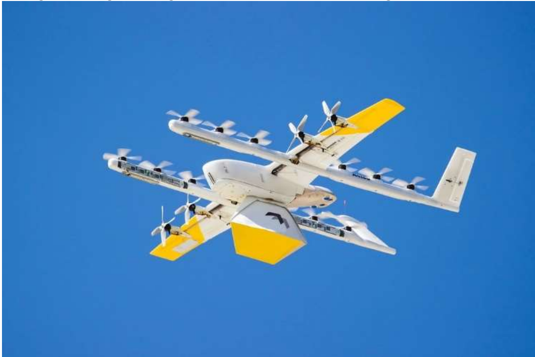
Figure 2. Wing Hummingbird Unmanned Aircraft with Package Attached
