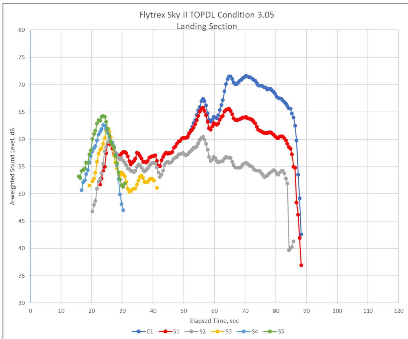
Figure 8. Sound Level Histories during TOPDL condition 3.05 – Landing
