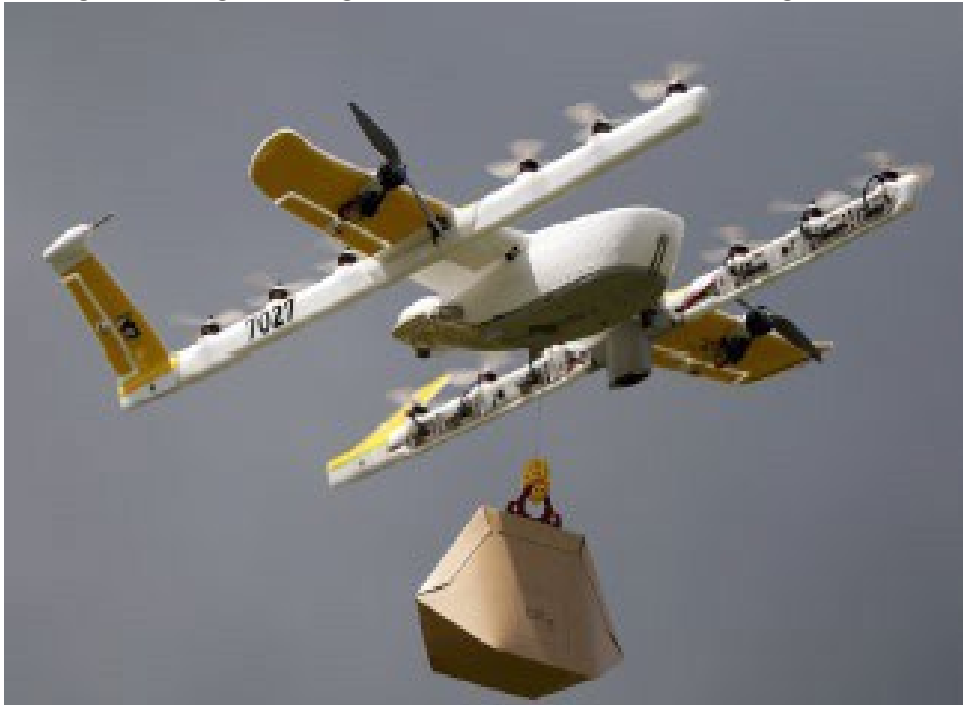
Figure 2. Wing Hummingbird Unmanned Aircraft with Package Attached
