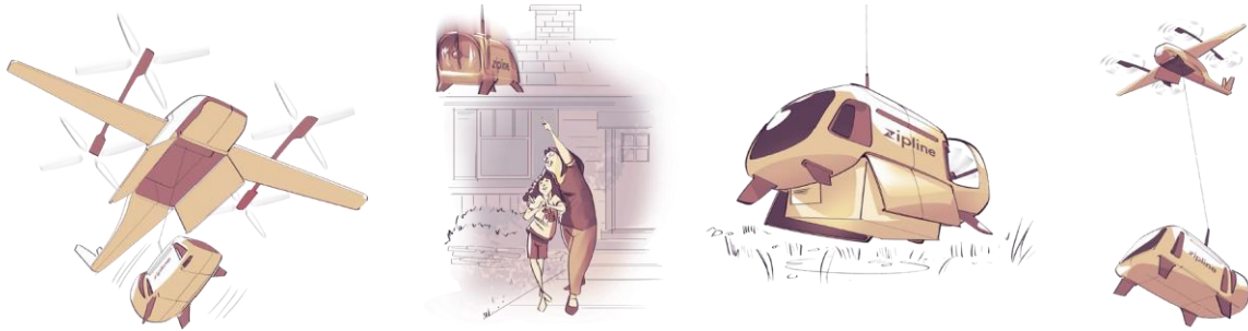
Figure 8. Droid softly delivers payload on intended surface and retracts back into P2 Zip
