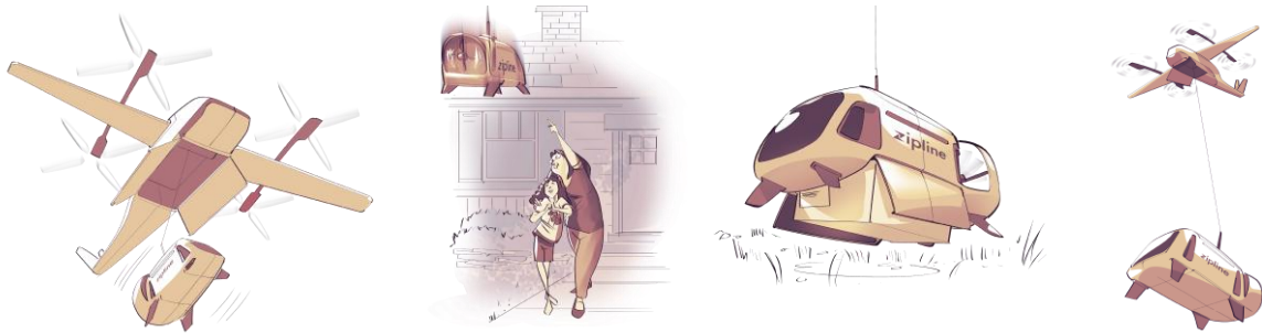
Figure 2.2-10. Droid softly delivers payload on intended surface and retracts back into P2 “Zip” UA
