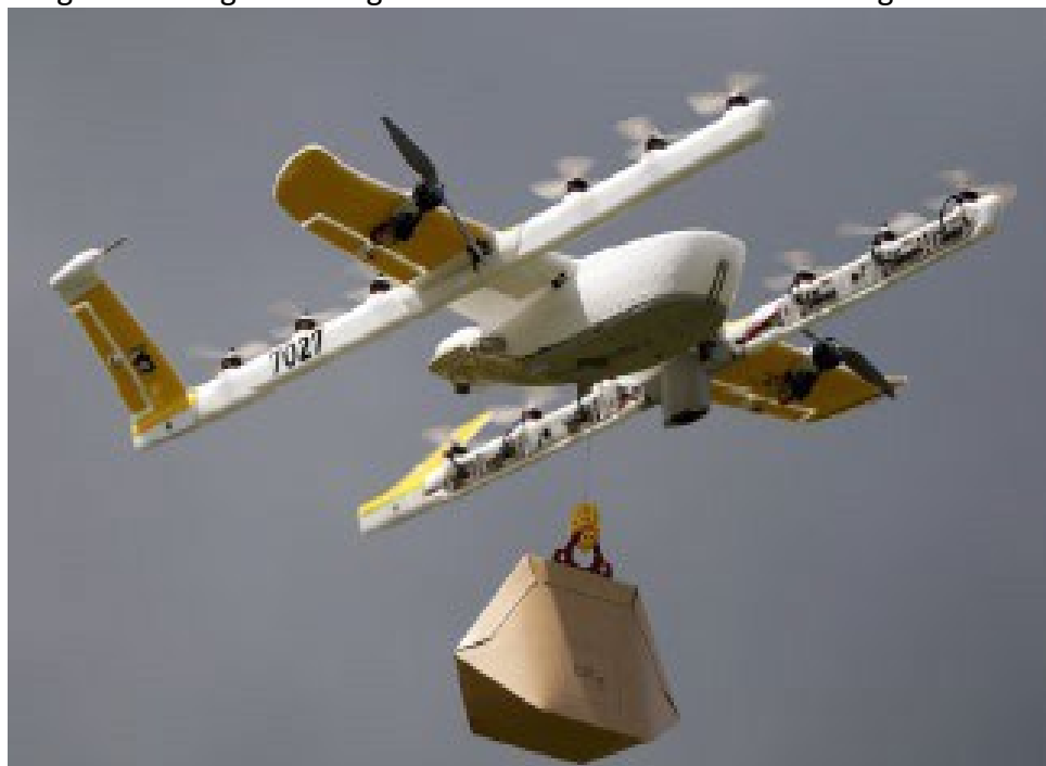
Figure 2. Wing Hummingbird Unmanned Aircraft with Package Attached
